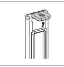
2) Align the hinge projection of the USB environmental protection cover on the guiding hole of the GOT. Put a supplied fixing screw through the hinge hole of the USB environmental protecting environmental.
