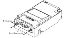
Turn the field network adapter unit upside down to check the fixing mechanism Loosen the two hexalobular socket screws until the fixing mecha nism is released
