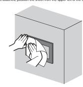
3) To attach the protective sheet, attach it from one direction gradually. Make sure to fit the protective sheet onto the joining surface closely without leaving any air between them.
