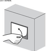
Peel the release paper off the back of the new protective sheet.
