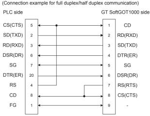
Cable Connection and Signal Direction
