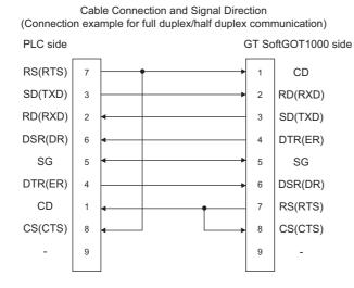
(2) Connection example which cannot turn ON/OFF CD signal (No. 1 pin) Connection example for exercising CD code control or DTR/DSR control.
