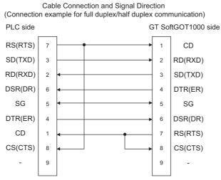
DC code control or DTR/DSR control is enabled by connecting the QC24 (N) to an external device as shown above.
