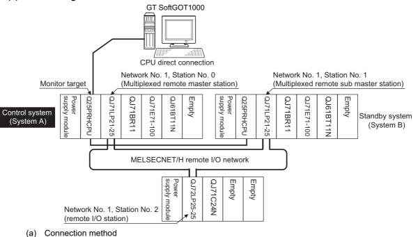
Connect the GT SoftGOT1000 and the control system PLC CPU (Q12PRHCPU, Q25PRHCPU) of the redundant system with an RS-232 cable or USB cable.
