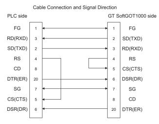
\* When performing a communication in the connection shown above, the CD signal is not required to be connected. For the RS-232C CD terminal check setting (set by the buffer memory address "10BH"), specify "without CD terminal check (writing "1")"
