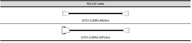
Use the cables to connect to the function extension board or function adaptor of MELSEC iQ-F and FXCPU. The following table shows the available communication types.
