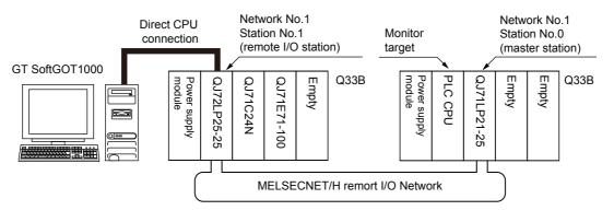
(a) Network modules in a remote I/O station The network units (QJ72LP25-25, QJ72LP25G, QP72BR15) of the remote I/O station are handled as PLC CPU.
