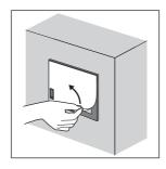
2. Peel the release paper off the back of the new protective sheet. With the protective film left on the sheet surface, attach the sheet on the GOT so that the USB environmental protection cover hole is just on the USB environmental protection cover of the GOT. For the protective sheet (covered USB environmental protection cover type), attach the sheet on the GOT so that the LED hole is just on the POWER LED section of the GOT.
