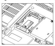
**5**. After the installation of option function board, attach the extension unit cover. (For installation of extension unit, install the extension unit.)
