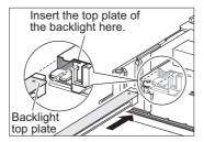
9. Connect the backlight cable connector to the GOT board connector. Do not put the cables of the backlight back to the cable holder A.Assemble the case in the reverse procedure of disassembly. (Tighten the fixing screws on the GOT rear face with a torque of 0.36 to 0.48 N•m).
