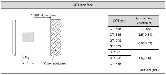
2. Select the option coefficient of the corresponding extension unit from the following list.
