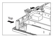
6. Remove the backlight cables one by one from the cable holder B.
