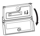
3. Press the CF card eject button, and then the button pops out.
