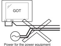
Bad example: The ground and power cables are installed together.
