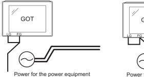
Good example: The ground and power cables are separated in wiring.
