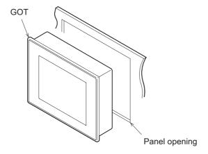
4. Place the mounting fixtures (included with GOT) on the mounting fixture attaching part of the GOT, and fix them by tightening the mounting screws in the torque range of 0.36 to 0.48N·m. (Failure to do so may distort the panel and make a surface waviness on the protective sheet.)
