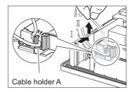
7. Pull out the backlight so that the backlight does not hit the packing.
