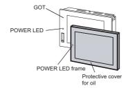
2. One corner of the cover is pulled outside, and it hangs it on the corner of the front panel of GOT.
