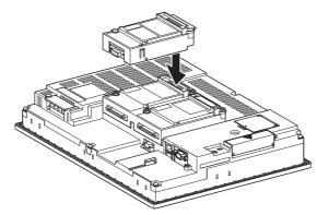
3. After installing the unit, fasten it by tightening the mounting screws (2 places) with tightening torque of 0.36 to 0.48N·m.
