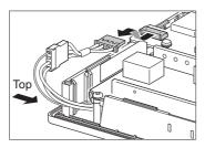
6. Remove the backlight cables from the cable holder A by pulling the backlight cables one by one in the arrow I direction and then in the arrow II direction.
