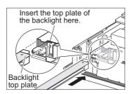
9. Connect the backlight cable connector to the GOT board connector. Secure the backlight cables with the cable holder B.Assemble the case in the reverse procedure of disassembly. (Tighten the fixing screws on the GOT rear face with a torque of 0.36 to 0.48 N•m).
