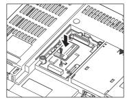
4. After the installation, tighten a fixing screw within the specified torque range (0.25 to 0.35N·m).
