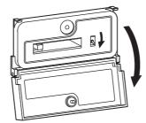
Insert the CF card into the CF card connector with the front side facing up.
