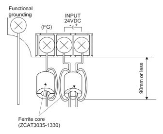
\* Be sure to ground the functional ground terminal and power FG terminal.
