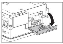
2. After confirming the battery is stored in the battery holder, insert the battery connector into the connector of the GOT.
