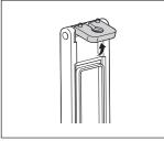
Tighten the screw with a torque of 0.36 to 0.48N•m. Fitting the hinge projections in the GOT guiding holes makes the cover installation work easier.
