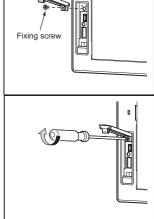
5. When the USB interface is used, unfix the latch to open the cover, and then connect the USB cable.
