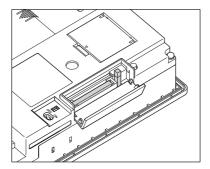
3. Push the CF card eject button of the GOT to lift the CF card and remove it.
