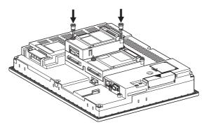
4. When installing another extension unit on the unit that has been installed, implement the above operations of step 1 to 3. When not installing an extension unit on the unit that has been installed, in order to avoid receiving electrostatic, stick accessory stickers to cover the top of mounting screws.
