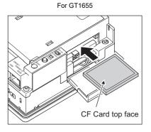
Close the cover of the CF card interface. Set the CF card access switch to ON.
