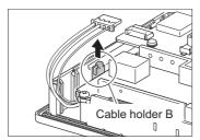
7. Pull out the backlight so that the backlight does not hit the packing.
