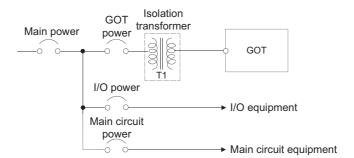
Twist 100V AC, 200V AC or 24V DC cable as closely as possible and connect the cable of the minimum length between modules.
