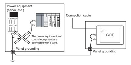
Do not connect the ground cables of the power equipment and control equipment with a wire.
