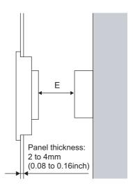
According to the dimensions in the following table, leave clearances between the GOT and the other devices. The values enclosed in square brackets apply to the case where no other equipment generating radiated noise (such as a contactor) or heat is installed near the GOT. However, keep the ambient temperature of the GOT to 55°C or lower.
