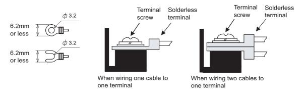
Applicable solderless terminal RAV1.25- 3, V2- S3.3, V2- N3A, FV2- N3A
