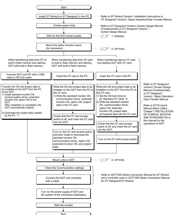
\* 1 By connecting with the Ethernet interface included as standard in GT 16, project data can be downloaded/uploaded. For download/upload of project data with the Ethernet connection, BootOS and standard monitor OS should be installed in the GOT in advance so that the GOT and PC can communicate with each other via Ethernet by setting Communication Settings. Refer to the following manual for details.
