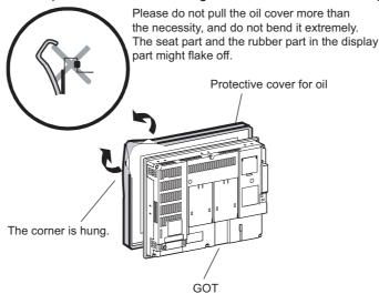
3. The oil cover was hung and the edge of the oil cover is sequentially obtained and obtain the oil cover to cover rubber packing parts in the back of GOT of the front panel. (It is the order of the arrow from A side to D side.)
