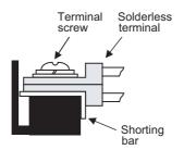
For the ground cable of the connection cable, use the following solderless terminals.
