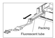
8. Install a new backlight so that its top plate is inserted between the metal parts of the backlight replacement hole. When inserting a new backlight into the backlight replacement hole of the GOT, make sure not to damage the sheaths of the cables. Insert the backlight all the way in.
