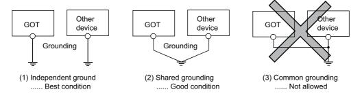
Use a cable of 2mm<sup>2</sup> or more for grounding when performing (1) or (2) above.
