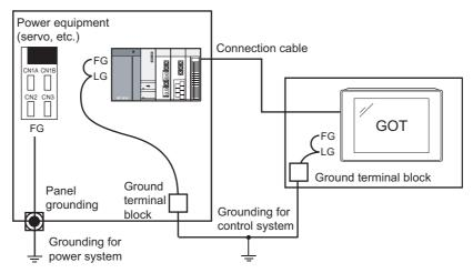
\* For the control equipment, ground the system at one end.
