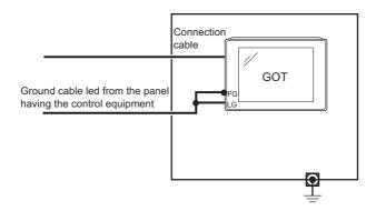
The malfunction occurred by the potential difference caused by the groundings in such a case, may be prevented by reducing the voltage with the following measure example 1, where the voltage is reduced.
