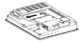
Install the option function board in the option function board interface.
