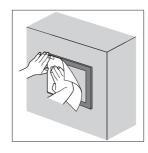
Make sure to fit the sheet on the GOT without wrinkles or air between the sheet and the GOT.
