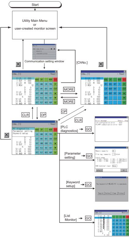
\*1 With setting special function switches (FX list monitor), the list monitor can be started on the monitor screen. When the list monitor is started on the monitor screen, the list editor cannot be used. For how to set special function switches, refer to the following.
