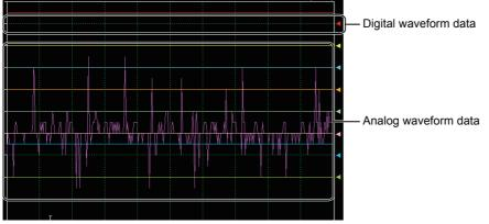
An arrow is displayed on the right edge of a digital waveform.
