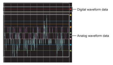
An arrow is displayed on the right edge of a digital waveform.
