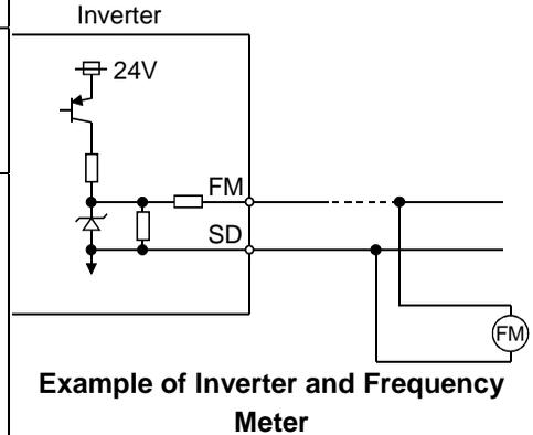
\*1. 0.5V or less when a DC ammeter of 300Ω or less internal resistance is connected to measure the output voltage.
