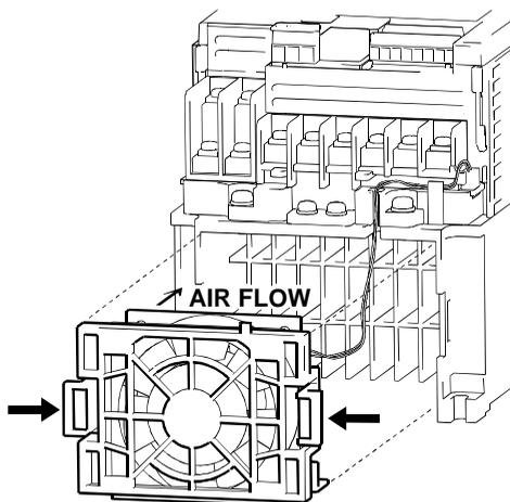
4) Remove the cooling fan and cooling fan cover.
