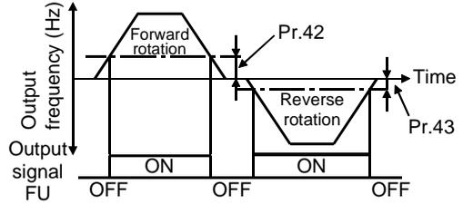
This function is effective for switching the timing of electromagnetic brake operation between forward rotation (rise) and reverse rotation (fall) during vertical lift operation, etc.
