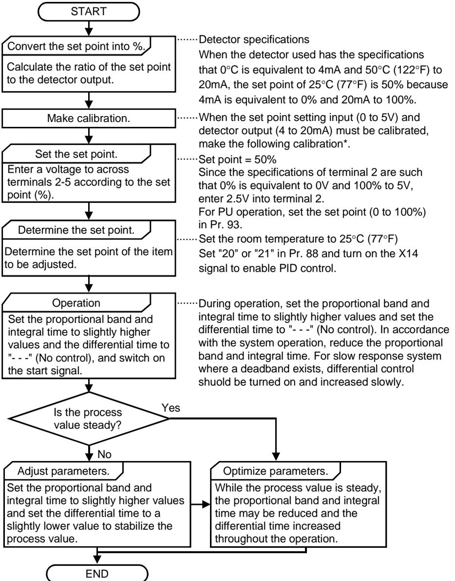
\*When calibration is required → Use Pr. 38 and calibration parameters C2 to C4 (terminal 2) and Pr. 39 and calibration parameters C5 to C7 (terminal 4) to calibrate the detector output and set point setting input. Make calibration in the PU mode when the inverter is at a stop.
