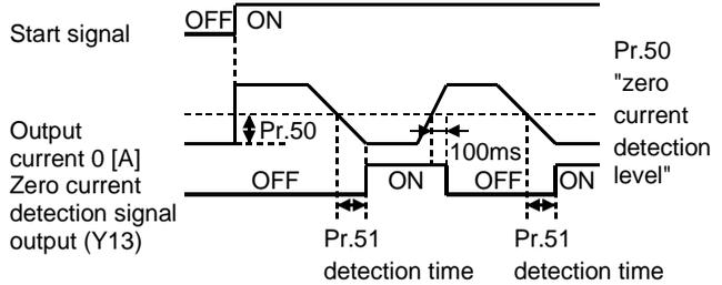
To prevent this, the output current "zero" signal can be output from the inverter to close the mechanical brake when the output current has fallen to "zero".
