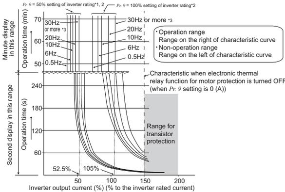
This function detects the overload (overheat) of the motor, stops the operation of the inverter's output transistor, and stops the output.
