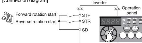
Operation example Operate at 30Hz.
