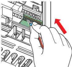
When using a single wire or a stranded wire without a blade terminal, push an open/close button all the way down with a flathead screwdriver, and insert the wire.
