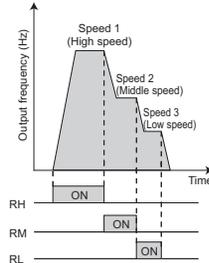
Operation example    Operation at high speed (60Hz)
