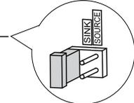
**Control logic switchover jumper connector**
