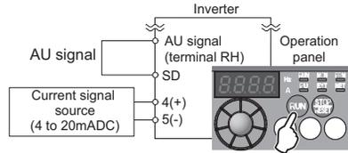
Operation example Operate at 60Hz.
