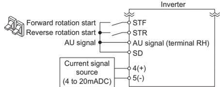
Operation example Operate at 60Hz.
