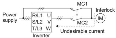
**(15) If the machine must not be restarted when power is restored after a power failure, provide a magnetic contactor in the inverter's input side and also make up a sequence which will not switch ON the start signal.**
