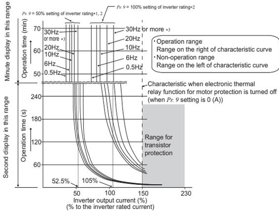
This function detects the overload (overheat) of the motor, stops the operation of the inverter's output transistor, and stops the output. (The operation characteristic is shown on the left.)
