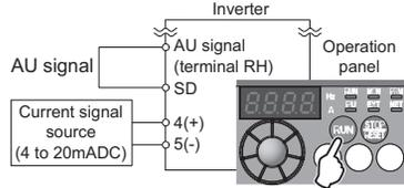
Operation example Operate at 60Hz.
