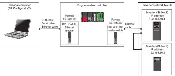
•When using FR-A800 with FR-A8NCG (FR-A800-GN) or FR-F800 with FR-A8NCG and setting the station number using the station number switches
