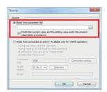
**4.** The setting can be changed for some parameters of the source inverter. To change the parameter setting value, enter the desired value in the setting value field. After the parameters of the source inverter are displayed in the list, the [<u>Convert...</u>] button in the "Convert" window will be active. Select [<u>Convert...</u>] to display the "Convert" sub window.
