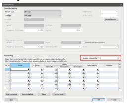
8. Click [Auto recognize]. The inverters connected with the personal computer are automatically detected.
