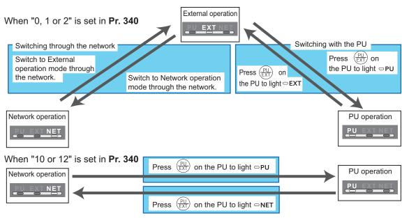
\*When using USB connection, operation mode changing is available from FR Configurator2. For the details of the operation mode switchover, refer to the Instruction Manual of the inverter.
