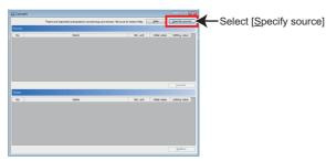
2. Select [Read from connected inverter]. Set the [Connection type], [Target station], and [<u>C</u>onnection setting], and click [<u>D</u>etection]. (When multiple inverters are selectable as the source inverter, the "Source inverter" window appears. Specify the model of the [Source inverter].) After detection, confirm the inverter model in the [Model] field, and click [OK]. The parameters are converted and the "Source" window closes.
