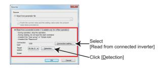
**3.** The setting can be changed for some parameters of the source inverter. To change the parameter setting value, enter the desired value in the setting value field. After the parameters of the source inverter are displayed in the list, the [<u>Convert...</u>] button in the "Convert" window will be active. Select [<u>Convert...</u>] to display the "Convert" sub window.
