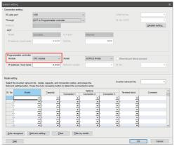
**11.** Click [Auto recognize]. The inverters connected with the personal computer are automatically detected.
