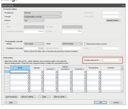
9. Click [Auto recognize]. The inverters connected with the personal computer are automatically detected.
