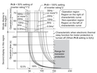
This function detects the overload (overheat) of the motor and shut off the inverter output by stopping the operation of the transistor at the inverter output side. (The operation characteristic is shown on the left.)
