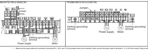
Connect the motor to terminals U, V, and W. The motor rotates counterclockwise when viewed from the motor load side when the forward rotation switch (signal) turns ON
