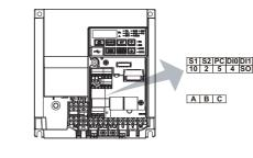
crimp terminals and stripped wire for the control circuit wiring. If only a single wire is used, the wire can be stripped and used without a ferrule.
