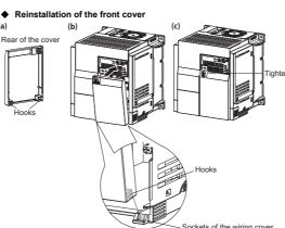
(b) Insert the hooks of the cover into the sockets of the wiring cover, and reinstall the
