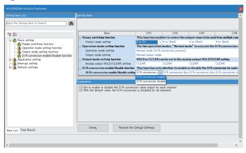
For the "Output range setting", check the input voltage specifications of the SCR (thyristor) and select from the following. Check the digital value and resolution of the output range, and set the upper/lower limit output limiter value of the manipulated value (MV).
