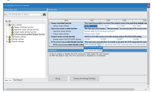
For the "Output range setting", check the input voltage specifications of the SCR (thyristor) and select from the following. Check the digital value and resolution of the output range, and set the upper/lower limit output limiter value of the manipulated value (MV).
