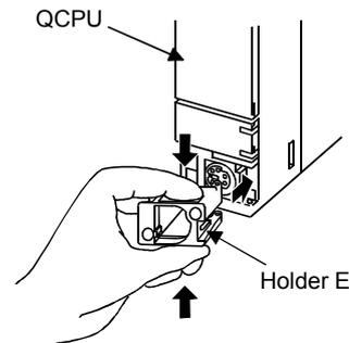
(3) Attaching Holder A and C or Holder B and D to the RS-232 cable
