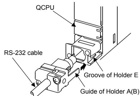
(5) Fixing Holder A and C or Holder B and D
