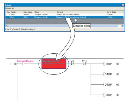
2. Check the corresponding error location and correct the error as instructed by the error/warning message.
