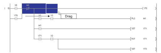
The columns are inserted. The screen image below shows the insertion of three columns.
