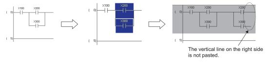
In such a case, set the range as shown below to copy or paste the elements.
