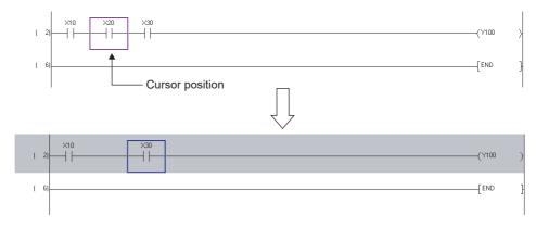
• In the 'Insert mode', contacts, coils, or application instructions newly input at the cursor position are inserted in front of the cursor.
