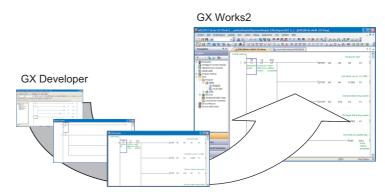
Therefore, GX Works2 can edit the sequence programs created by GX Developer, making it possible to utilize program assets effectively.
