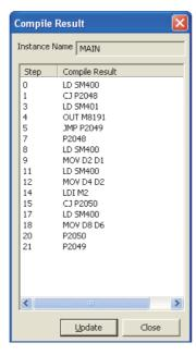
The compilation result is not displayed when the compilation target is an assignment command in which the source data and the target data are the same. Example in Structured Text: M0 :=M0;
