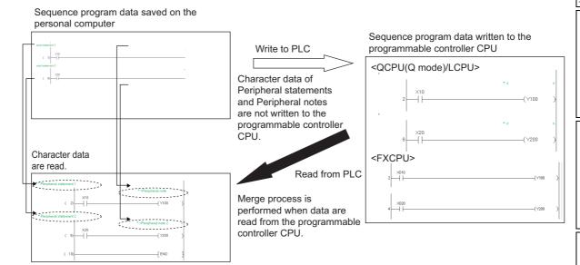
The following table shows the different process status with the execution of the merge process when reading programs from the programmable controller CPU.
