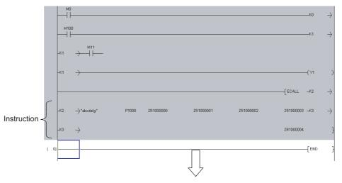
Create the wrapping source symbol (->) in the line ②, and create the wrapping destination symbol (>-) in the line ③.
