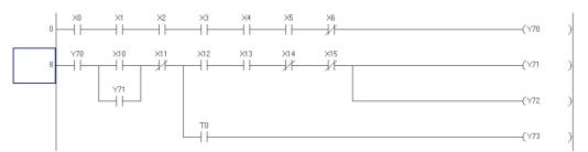
For selecting multiple ladder blocks, specify the range by dragging the cursor down from the start position of cut or copy.
