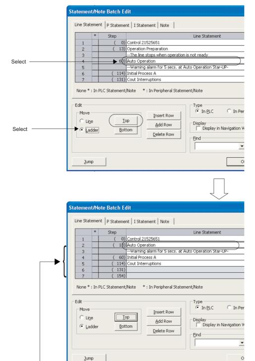
The unit of line statements of ladder block above the selected statement is deleted, and the selected statement below the cursor position moves one ladder block upward.
