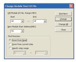
For FXCPU, "Old Module I/O No. Range (HEX)" is indicated as "Old Module I/O No. Range (0 - 7)", and "New Module Start Address (HEX)" is indicated as "New Module Start Address (0 - 7)".
