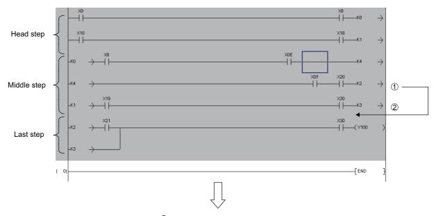
Insert a new line to 3, and create the wrapping source symbol (->) with K5 and wrapping destination symbol (>-) with K3.
