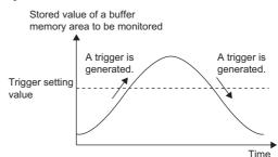
(3) Post-trigger logging points When the set points of data is collected after a hold trigger is generated, the logging operation is stopped.
