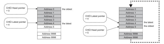
The head pointer does not change (fixed to 0) until CH1 Logging data (Un\G10000 to Un\G19999) becomes full after the logging start.
