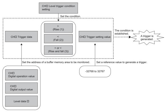
To generate a hold trigger when a value in CH1 Digital output value (Un\G400) is greater than 10000, set as follows.
