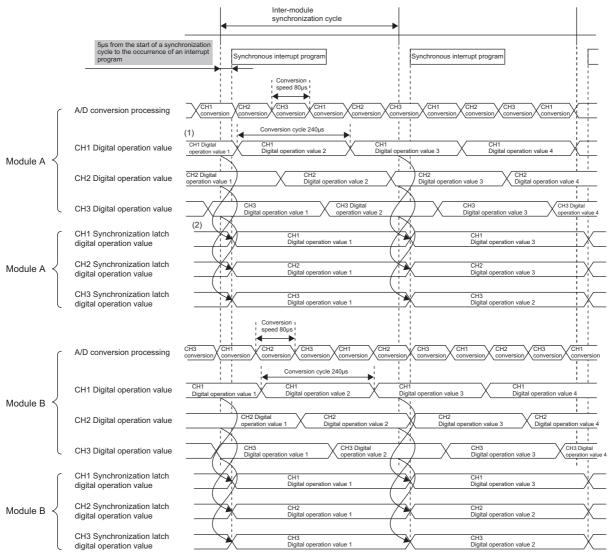
(1) CH Digital operation value is stored in the A/D converter module according to the conversion speed.
