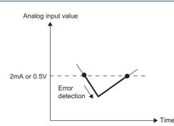
The setting for 'CH1 Input signal error detection setting value' (Un\G529) is ignored.
