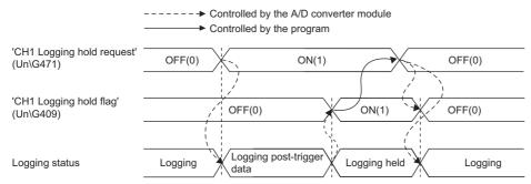
Logging does not stop when 'CH1 Logging hold request' (Un\G471) is changed from on to off before ON (1) is stored in 'CH1 Logging hold flag' (Un\G409).
