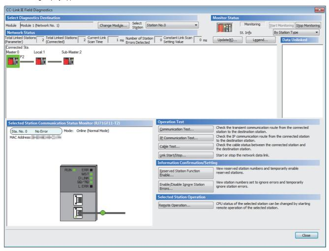
If an error icon appears in "Network Status" area on the "CC-Link IE Field Diagnostics" window, use the CC-Link IE Field Network diagnostics to identify the cause of the error and take corrective actions. (SP Page 269 Checking the Network Status)
