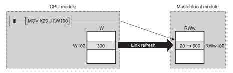
• Good example (In addition to direct access, writing the same data to the CPU module device) The value written by direct access is reflected.
