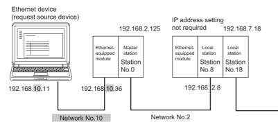
O not use the third octet (network number) of the IP address same as that of other network modules and other CPU modules using the IP packet transfer function.
