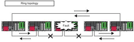
The system disconnects faulty stations and automatically performs loopback to continue the data link.
