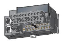
Loosening the terminal block mounting screws (two points) allows the two-piece terminal block to lift and be removed.
