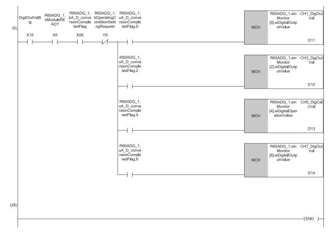
(0) CH1 Digital output value, CH3 Digital output value, CH5 Digital operation value, and CH7 Digital output value are to be read.
