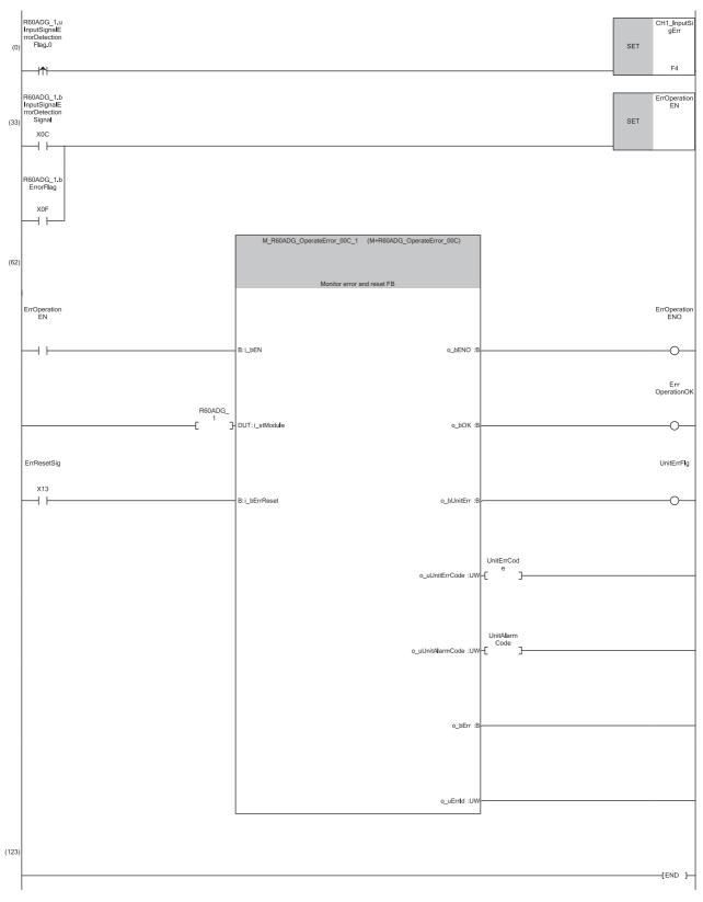
(0) The processing at the time when an input signal error is detected in CH1 is to be performed.
