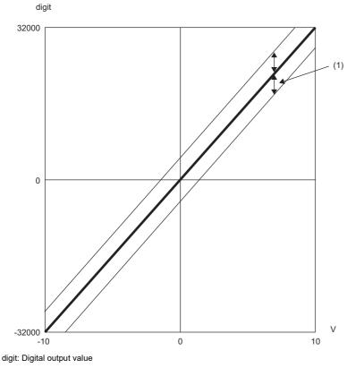
digit: Digital output value V: Analog input voltage (V) (1) Voltage fluctuation range
