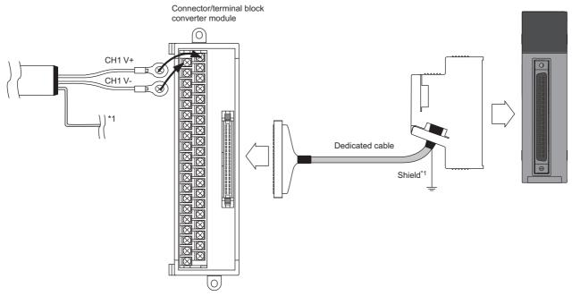
\*1 Be sure to use a shielded cable. The shield must be grounded.
