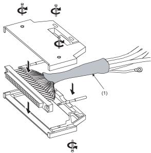
(1) Cover the cables on which a conductive tape has been applied with a heat-shrinkable tube.
