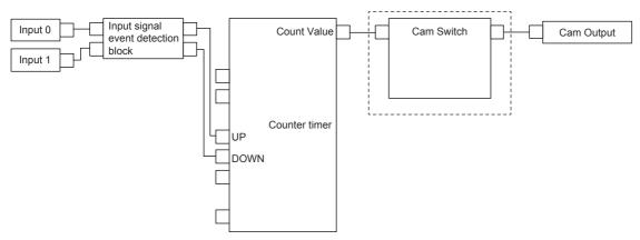
Create the hardware logic by using a cam switch block, as shown in the dotted line frame.
