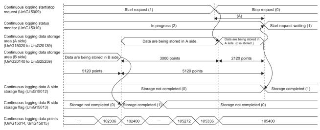
(A) Even though the stop request is issued, continuous logging does not stop immediately. Continuous logging stops when the data for 5120 points has been stored in Continuous logging data storage area in which data is being stored.
