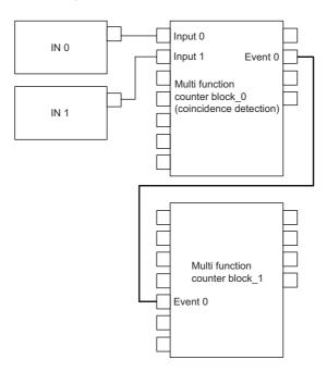
• Multi function counter block \_0 detail window (coincidence detection)
