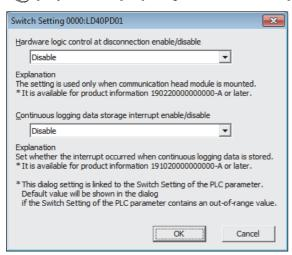
When the own station is disconnected, the operations of the flexible high-speed I/O control module differ depending on the setting of "Hardware logic control at disconnection enable/disable" in the switch setting or that of "Error Time Output Mode" in the intelligent function module detailed setting. For details, refer to the following.
