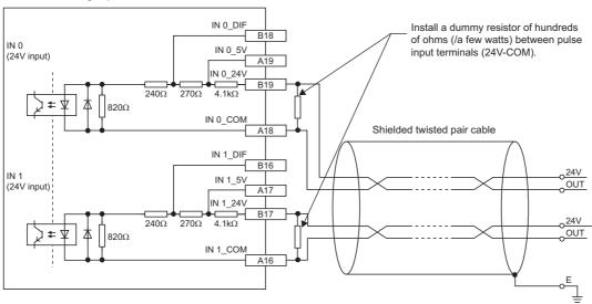
The following example describes how to select a dummy resistor (how to calculate a resistance constant and rated power of a dummy resistor).
