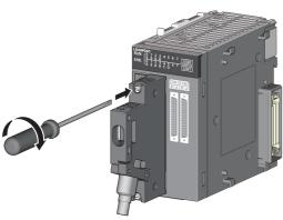
**2.** Tighten the two connector screws (M2.6).
