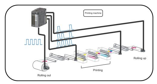
The ratio (x/y) used in ratio conversion must be " $y \ge x$ " when a signal multiplied by x/y is output to an input signal. Conversions with the ratio exceeding one time cannot be performed.
