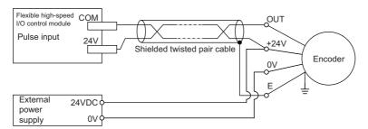
• Do not wire the module and an encoder as shown in the figure below. Because a current flows through a shielded twisted pair cable in a single direction and the canceling effect disappears, the module is easy to be affected by electromagnetic induction.
