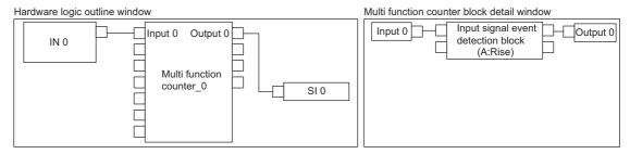
• For the linking of the multi function counter block detail window (Counter\_0(16bit\_Unsigned)), a value other than 0 is recommended for "Compare Value". If 0 is set in "Compare Value", an interrupt request is output to the CPU module when the operation of the hardware logic starts (when the count value starts to be counted from 0).
