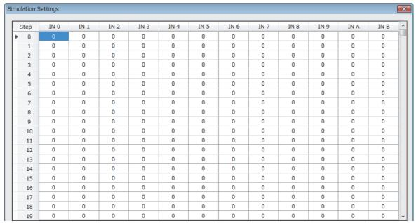
**2.** Click each cell in the external input signal data setting area and switch "0: External input signal OFF" and "1: External input signal ON". By default, "0: External input signal OFF" have been set in all cells.
