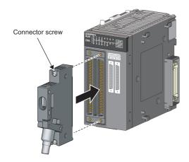
**1.** Plug the connector into a slot on the flexible high-speed I/O control module.
