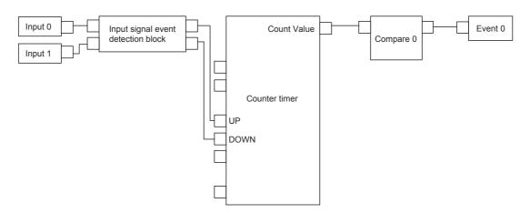
The multi function counter block\_0 counts external input signals. When the count value becomes equal to the compare value, an event signal is output to the multi function counter block\_1.
