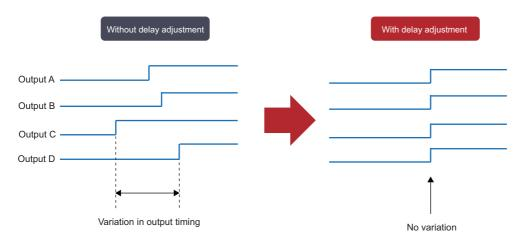
The timing variation due to electronic components can be adjusted.
