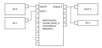
Multi function counter block \_0 detail window (coincidence detection)
