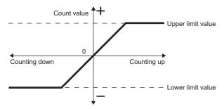
If "Count Value" has reached the upper limit value in up count, "Count Value" does not change in the next up count and the overflow error (error code: 100 $\square$ H) occurs. "Count Value" does not change until the preset function is performed even if down count is performed.
