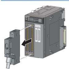
**1.** Loosen the two connector screws and pull out the connector from the module.
