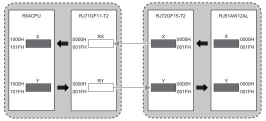
The following shows the correspondence between CPU module devices and I/O signals of the RJ51AW12AL.
