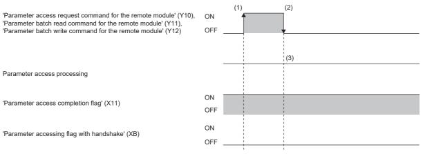
(1) Turn off and on any of the signals at any time to start the parameter access
