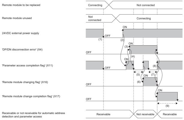
(1) Turn off the 24VDC external power supply connected to the RJ51AW12AL.
