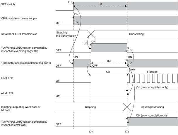
(1) While holding down the SET switch, reset the CPU module or power off and on the system. (Hold down the SET switch for one second or longer.)
