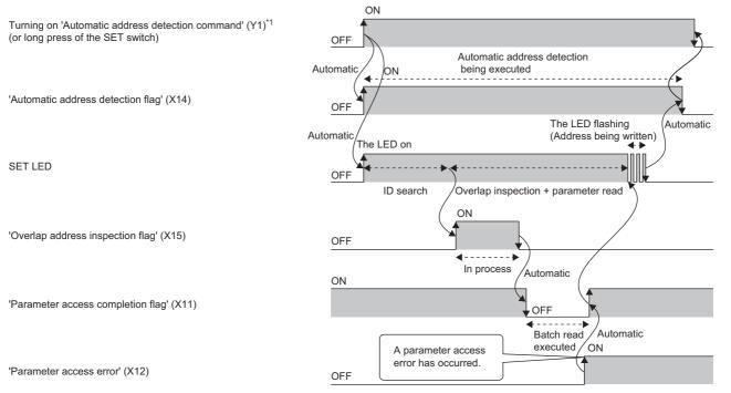
\*1 After turning on 'Automatic address detection command' (Y1), check that 'Automatic address detection flag' (X14) is on or check the SET LED status. Then, turn off 'Automatic address detection command' (Y1) with a program.
