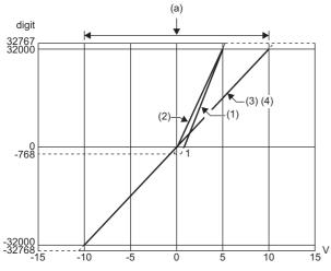
digit: Digital output value V: Analog input voltage [V]
