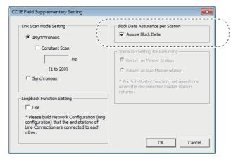
• Do not set the parameter using the CCPASET instruction in the master station. Correct operation of the multiple input module cannot be guaranteed because the module operates with the block data assurance per station disabled when the CCPASET instruction is executed. (The CCPASET instruction is intended to configure parameters for a master/local module. For details on the CCPASET instruction, refer to the user's manual for the master/local module used.)
