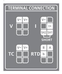
V: At current input and micro voltage input I: At current input TC: At thermocouple input RTD: At resistance temperature detector input
