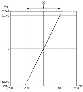
digit: Digital output value mV: Analog input voltage [mV] (a) Practical analog input range
