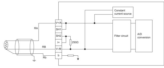
Install a resistance temperature detector so as to shorten the wiring length (minimize the conductor resistance values of RA, RB, and Rb) and set each conductor resistance value of RA, RB, and Rb to 150Ω or less. An accuracy error occurs with the following ratio by 1Ω conductor resistance value.
