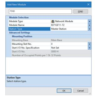
**5.** Click the [OK] button in the following window to add the module labels of the master/local module.
