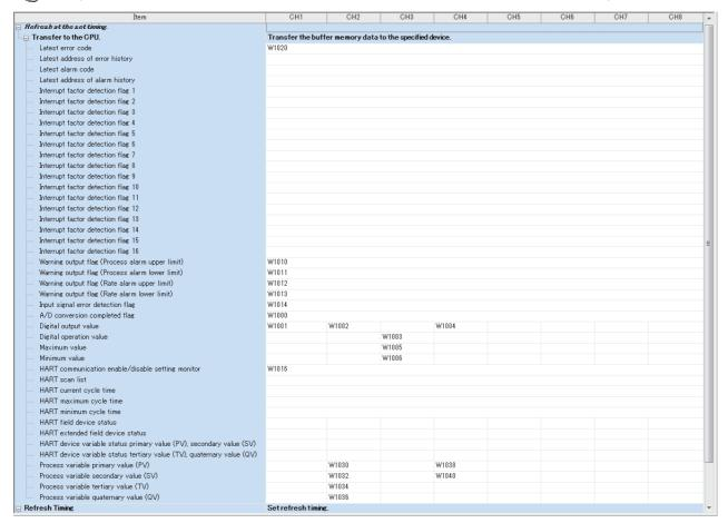
**8.** Write the set parameters to the remote head module on the intelligent device station. Then reset the remote head module or power off and on the system.
