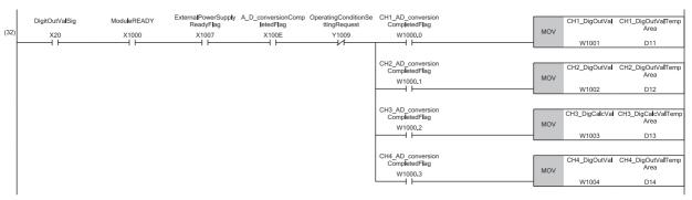
(32) Reads values of CH1 Digital output value, CH2 Digital output value, CH3 Digital operation value, and CH4 Digital output value.
