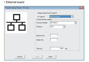
4. Set the details of "Communication setting" corresponding to the selected "PC side I/F".
