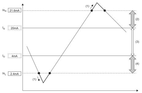
In<sub>H</sub>: Input signal error detection upper limit value
