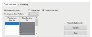
2. Enter a positioning data number to be executed in "Positioning data No."
