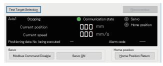
The test target can be changed in the "Select test target" screen by clicking the [Test Target Selection] button on the "Positioning test" screen.
