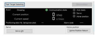
The test target can be changed in the "Select test target" screen by clicking the [Test Target Selection] button on the "Positioning test" screen.
