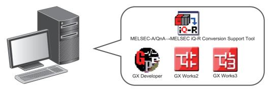
MELSEC-A/QnA→MELSEC iQ-R Conversion Support Tool, GX Developer, GX Works2, and GX Works3 are required.
