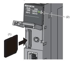
**1.** Insert an SD memory card (1) straight into the SD memory card slot with its cutout pointed down.
