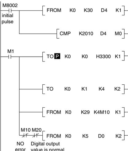
The ID code for the special function block at position "0" is read from BFM #30 of that block and stored at D4 in the main unit.
