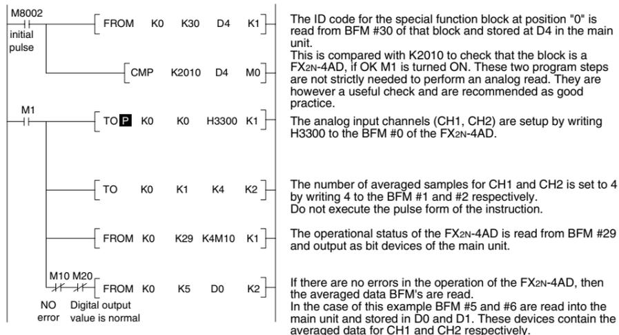
The ID code for the special function block at position "0" is read from BFM #30 of that block and stored at D4 in the main unit. This is compared with K2010 to check that the block is a FX2N-4AD, if OK M1 is turned ON. These two program steps are not strictly needed to perform an analog read. They are however a useful check and are recommended as good practice.
