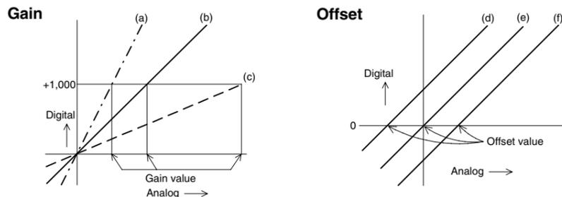
Gain determines the angle or slope of the calibration line, identified at a digital value of 1000.
