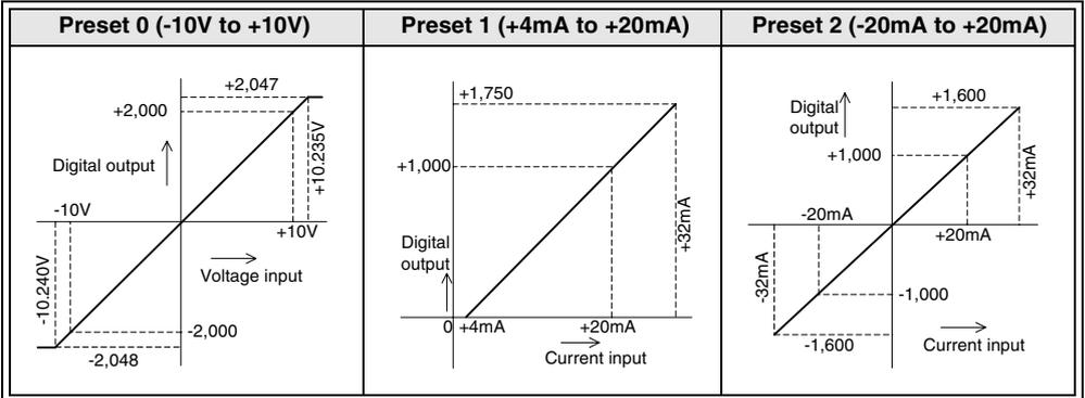
NOTE: Preset ranges are selected by an appropriate setting in the buffer memory of the analog block. Current/Voltage input selection must match the correct input terminal connections.
