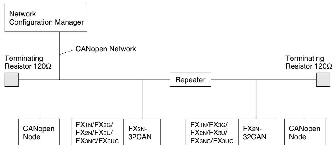
Network Manager Node:Station which controls the data link system
