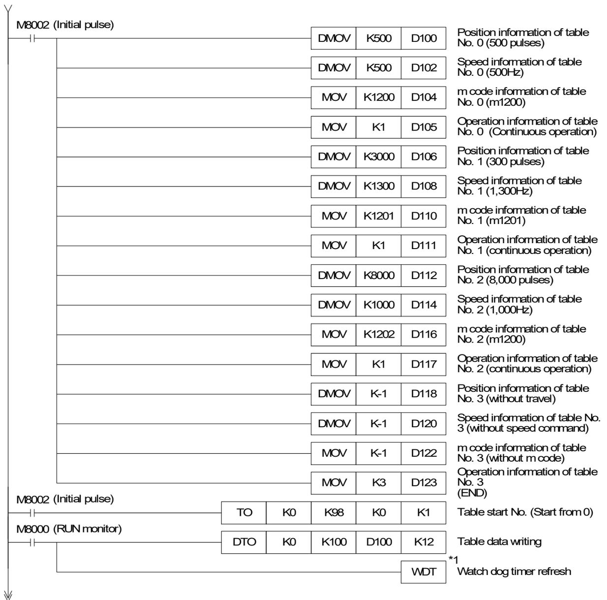
\*1 If any FROM/TO commands are used for many buffer memories at the same time, an watch dog timer error will occur.
