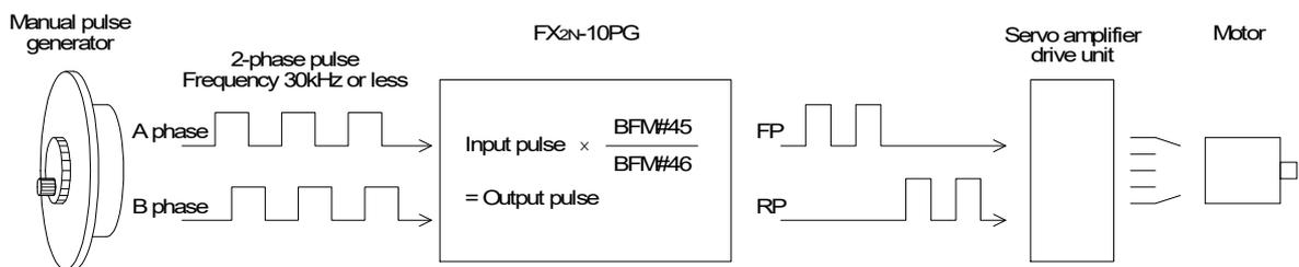
The output pulse (frequency and pulse amount) of FX2N-10PG is gained as follows:
