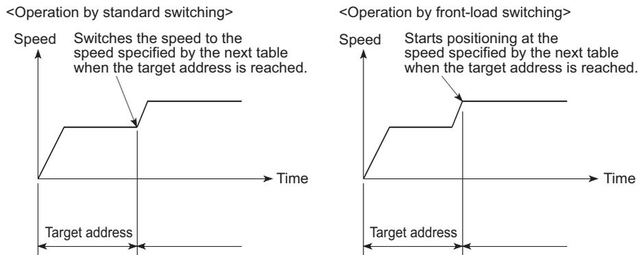
**8.9.4 Operation example 2 (position-to-speed operation)**
