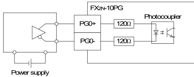
2) When NPN open collector transistor is used
