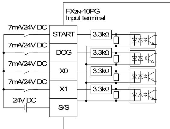
2) When NPN open collector transistors are used
