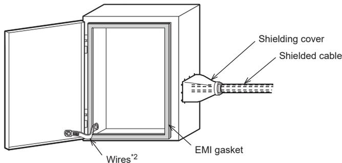
\*2 This wire is used to improve the conductivity between the door and control cabinet.
