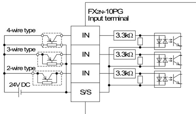
Reread **IN** terminal as START, DOG, X0 or X1 according to the application.
