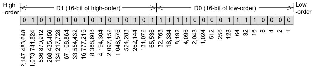
32-bit data is represented by a group of data registers with adjacent numbers. (The high-order bits are larger numbers and the low-order bits are small numbers.)
