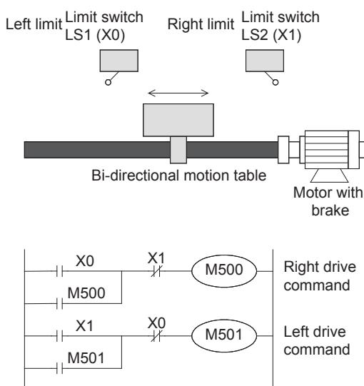
In some cases, it is required to move the positioning table in the same direction after power failure.
