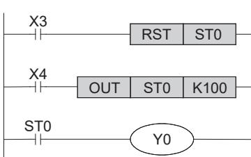
The timer ST0 starts timing at the moment X4 changes to ON. The timer keeps its current value if X4 is set to OFF or if the power is turned off during timing.
