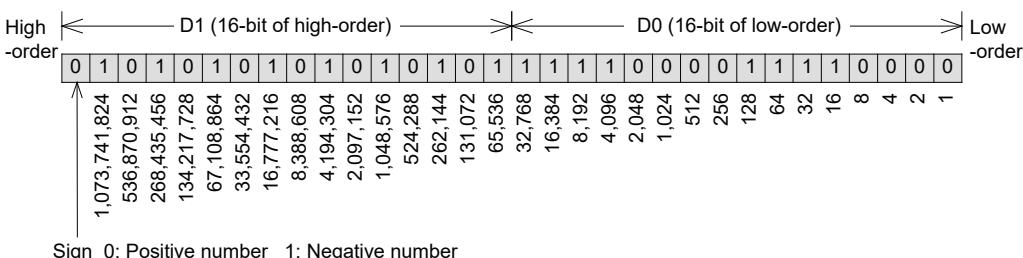
32-bit data is represented by a group of data registers with adjacent numbers. (The high-order bits are larger numbers and the low-order bits are small numbers.)
