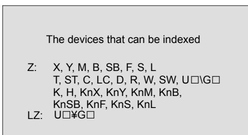
The main devices that can be indexed with index registers are those listed on the left. The devices on the left are used in the instructions.
