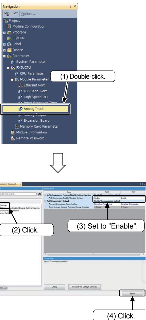
(1) Double-click [Parameter] → [FX5UCPU] → [Module Parameter] → [Analog Input] on the navigation window.
