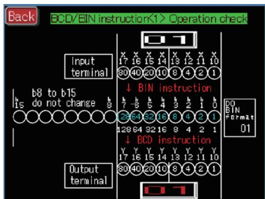
BIN instruction..... When the drive input is ON, the BCD value of the transfer source is converted to BIN and transferred.
