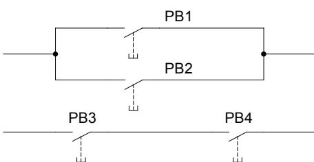
An input switch always connected in parallel or an input switch used as a serial connection can each be handled as one input.
