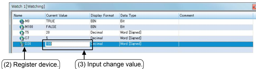
(1) Open the Watch Window. Refer to the previous section "Watch Window" for details on opening the window.
