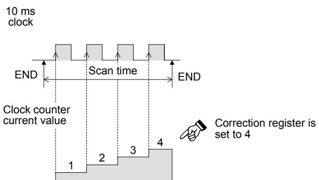
The correction register updates and stores the latest value of the clock counter at every interval.
