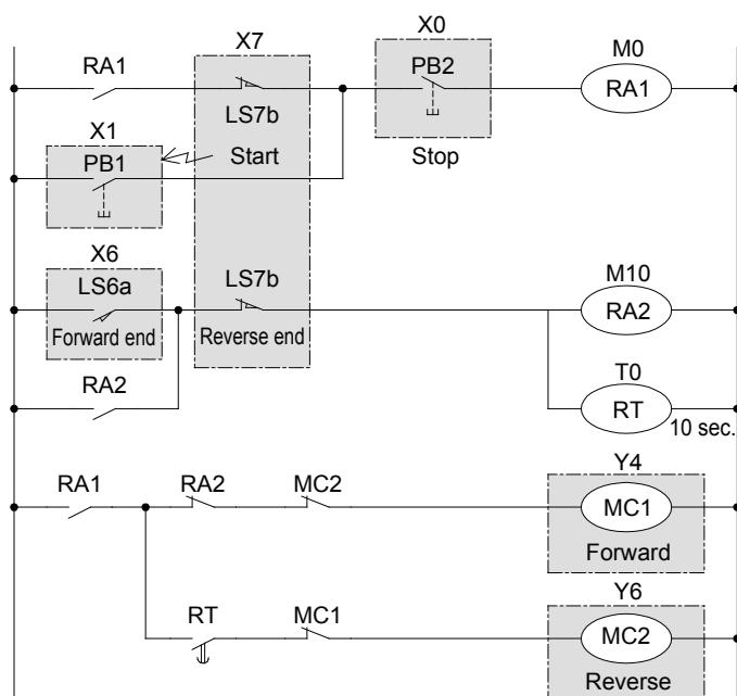
In addition to the input/output relays, the timer RT and controller relays RA1 and RS2 are assigned to T0, M0 and M10.
