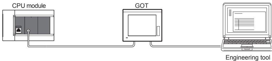
Complete the settings for communicating with the FX5U CPU module using the GOT (direct connection) transparent connection.
