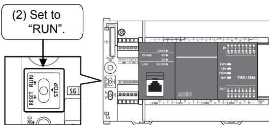
(1) It is assumed that the ladder program (sequence program) has been written to the CPU module, and the PLC has been reset or the power turned OFF and ON prior to this operation.
