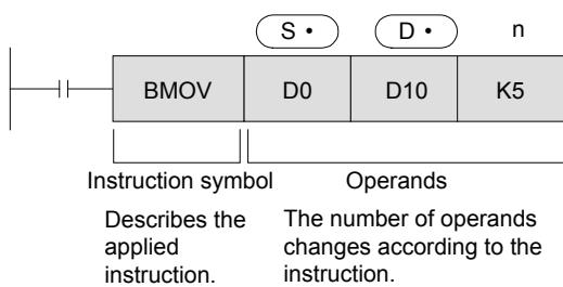
**S •**: The so-called source is the operand which does not change according to the execution of the instructions.
