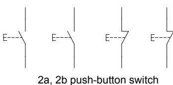
When a pushbutton switch has 2a, 2b contacts as shown on the left, the PLC needs one input for the 1a or 1b contact.
