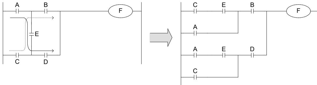
A circuit in which current flows in both directions must be rewritten as shown above. (The circuit when having no D, and the circuit when having no B, in parallel. It was connected.)
