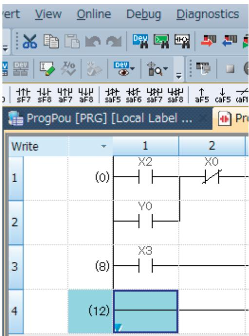
(2) The ladder program is converted. When the conversion processing is completed and the input ladder blocks are finalized, the color of those ladder blocks changes from gray to white.
