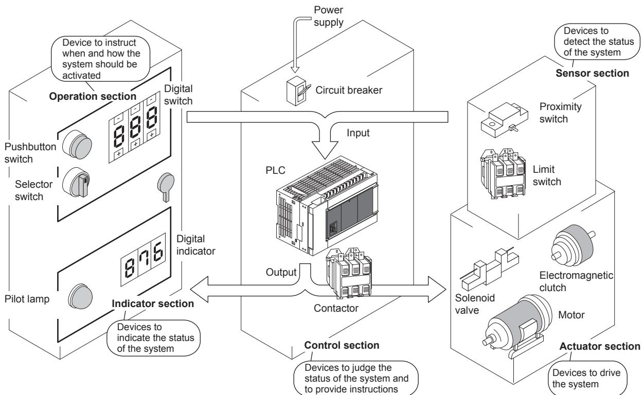
The PLC is activated by **command inputs** such as inputs from pushbutton switches, selector switches and digital switches located at the operating panel, and by **sensor inputs**, such as inputs from limit switches, proximity switches and photoelectric switches, which detect the status of the system, in order to control **drive loads** such as solenoid valves, motors and electromagnetic clutches, and **indication loads** such as pilot lamps and digital indicators.
