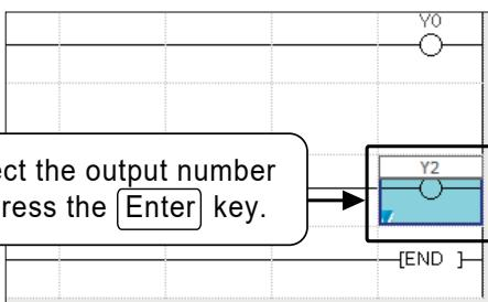
(2) The device can be modified. Modify the device to "Y2", and press the **Enter** key.
