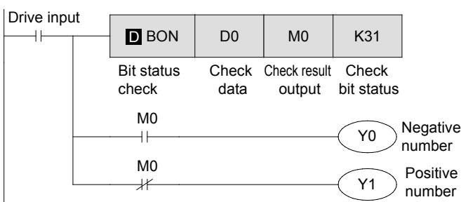
When the 31st bit (highest bit) of the 32-bit data D1 and D0 is ON, M0 is turned on.
