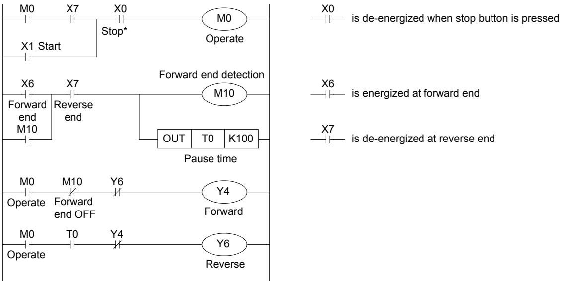
\* A N.C. contact (normally closed contact) is used for the stop button PB2, so the N.O. contact (normally open contact) is used on the sequence circuit.
