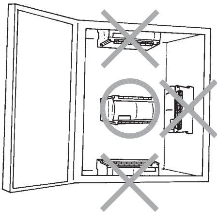
The PLC can be directly mounted onto the control panel using the mounting holes on the four corners, or directly mounted onto a DIN rail.
