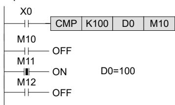
When the output result directly starts from the bus line as shown in the left diagram and the drive input X0 is turned off, the output M11 remains ON without regard to changes in D0.
