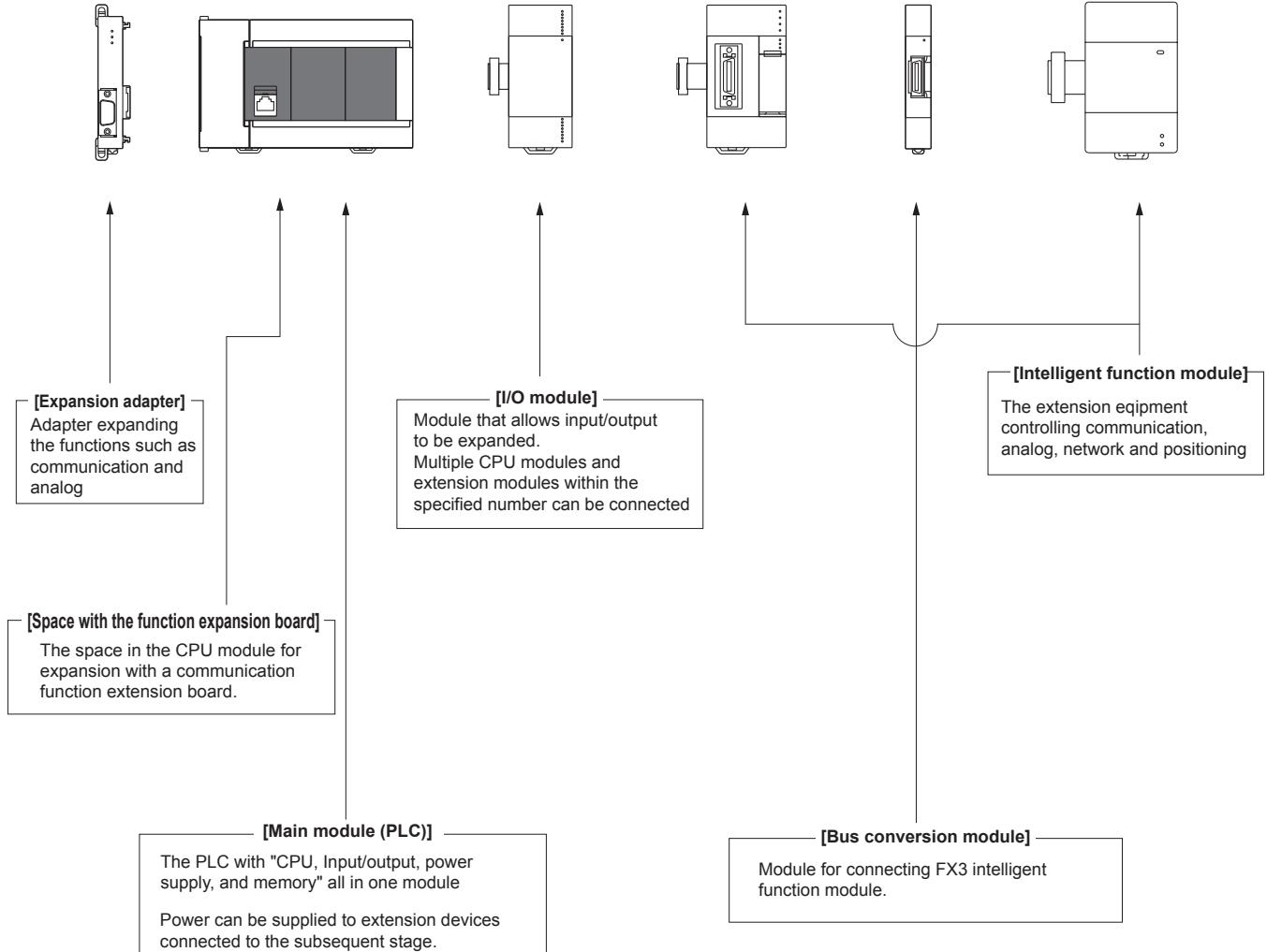
The types and the number of the equipments that can be connected depend on the series and the model name of the CPU module.
