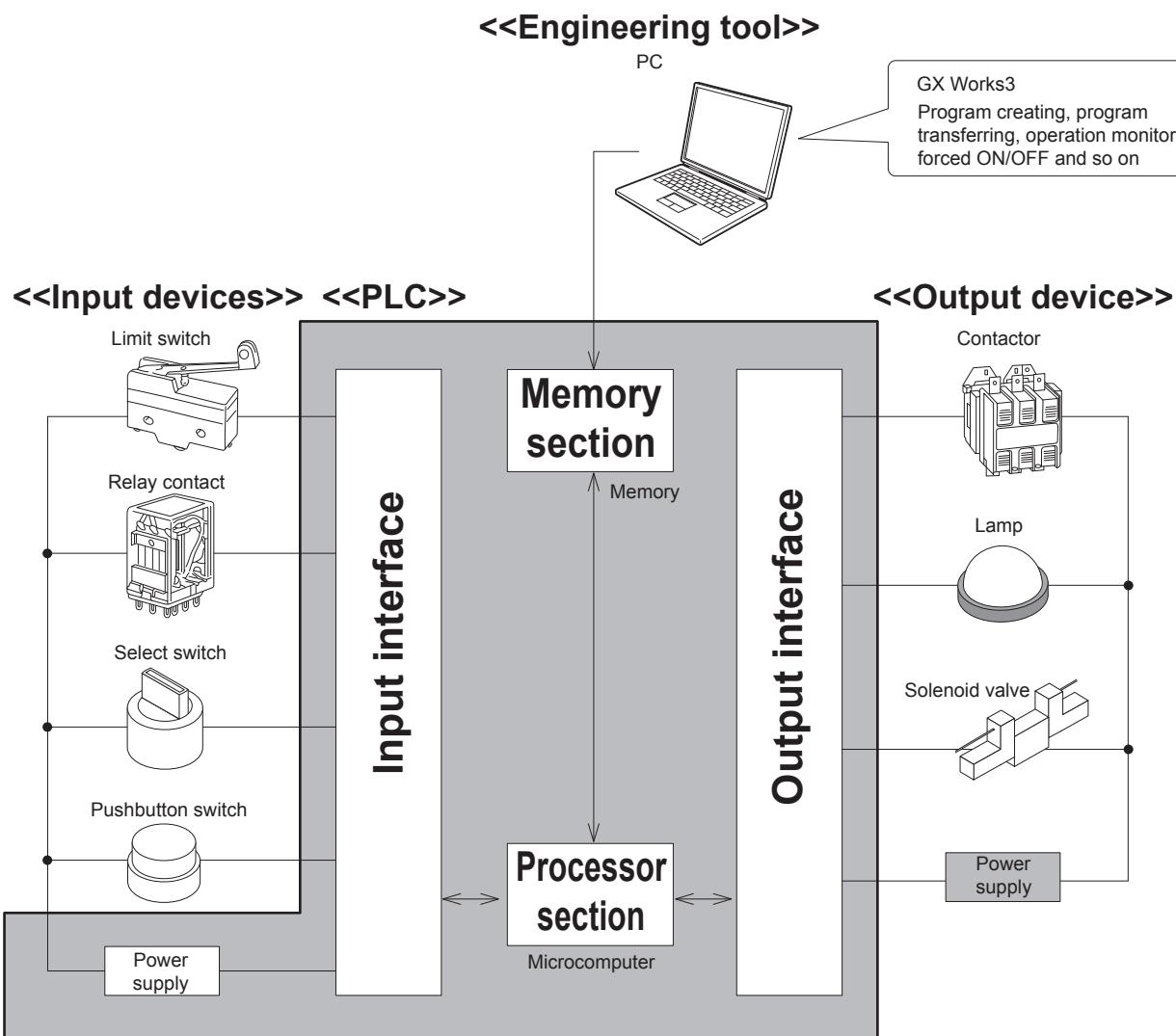
A PLC incorporates an electrical circuit mainly comprised of a microcomputer and memory. Input/output interfaces exist between input/output devices and the electronic circuit to connect them. The engineering tool is used to write a program to the memory in the PLC.
