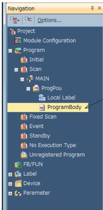
Double-click [Program] → [Scan] → [MAIN] → [ProgPou] → [Program Body] on the navigation window. The sequence circuit diagram will appear.
