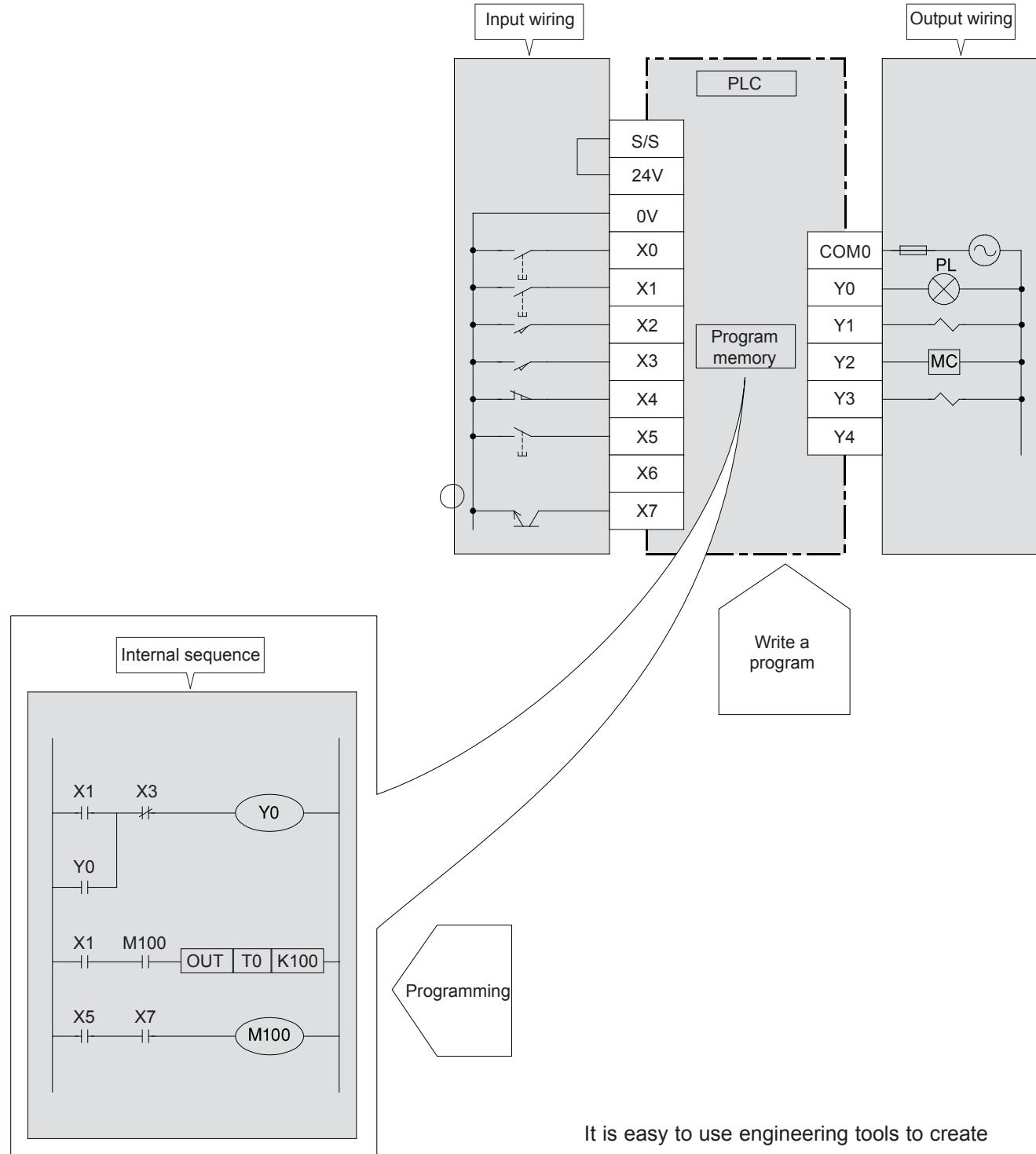
It is easy to use engineering tools to create the internal sequence program, which is equivalent to internal PLC wiring.
