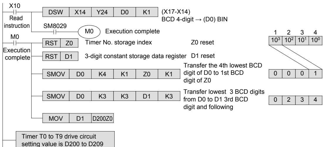
The **SMOV** instruction handles BIN data, but when this instruction is used, the data is automatically converted to BCD. Each BCD digit is moved, before it is returned to a BIN value.
