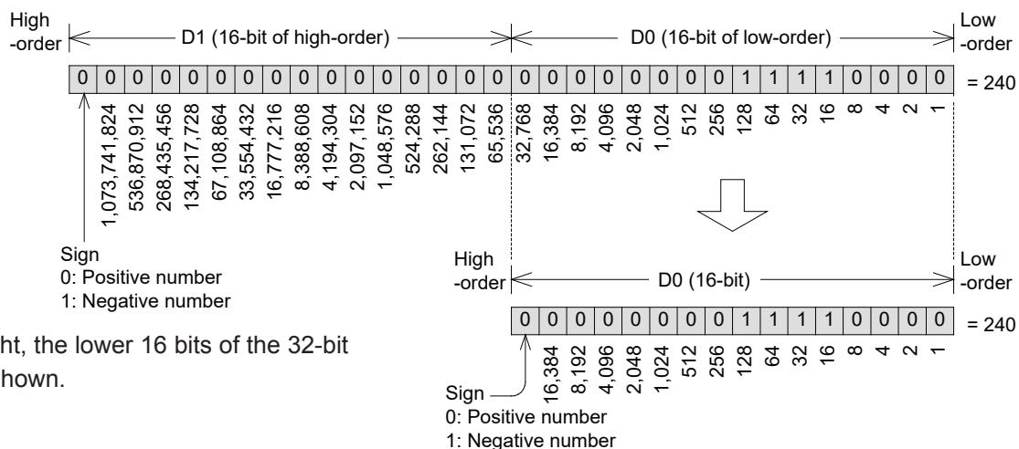
On the right, the lower 16 bits of the 32-bit data are shown.
