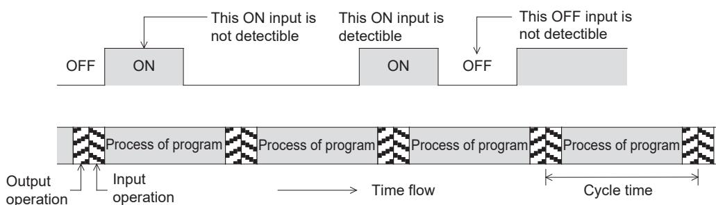
In principle, the widths of input pulses (ON and OFF inputs) for a PLC must be longer than the cycle time of the PLC.
