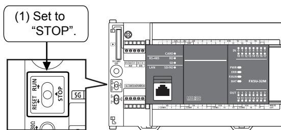
(1) Set the "RUN/STOP/RESET" switch of the CPU module to "STOP".
