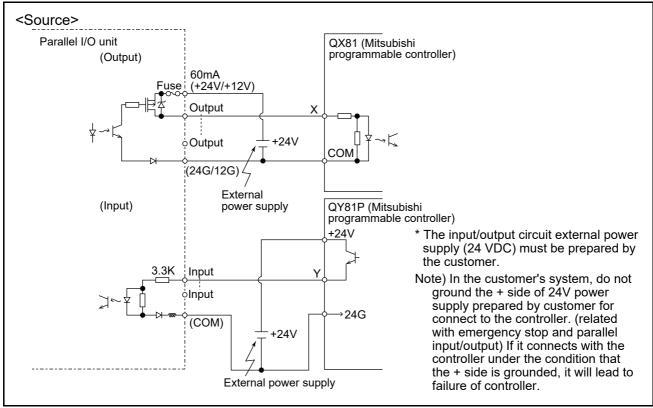
Fig.3-37: Connection with a Mitsubishi PLC (Example of source type)
