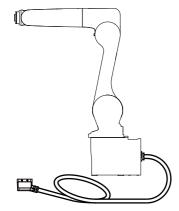
The fixed type machine cable can be used instead of the supplied one (5 m) to extend the distance between the controller and the robot.
