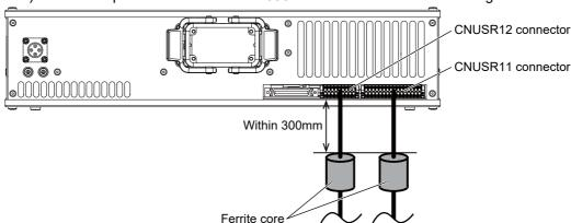
Fig.3-6: Installation position of ferrite cores
