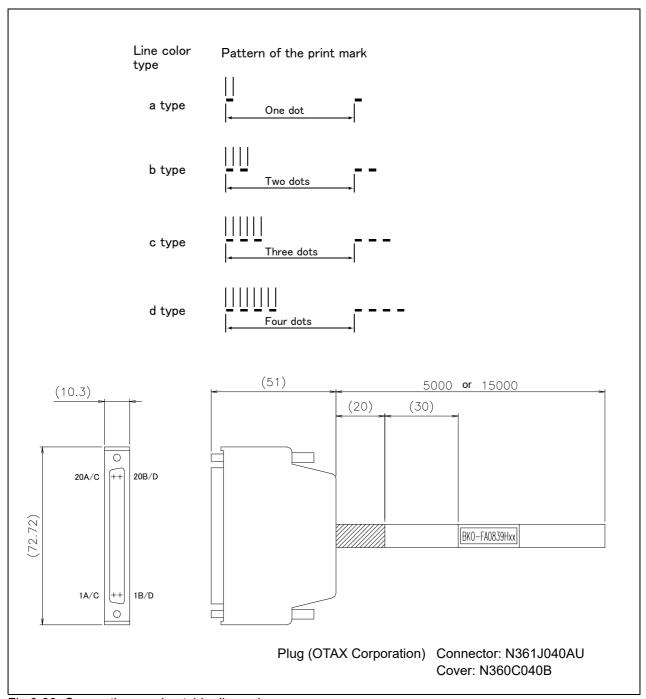
Fig.3-30: Connections and outside dimensions
