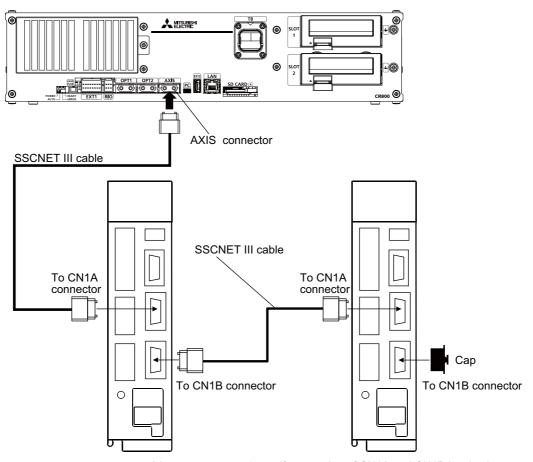
\* It cannot communicate, if connection of CN1A and CN1B is mistaken.
