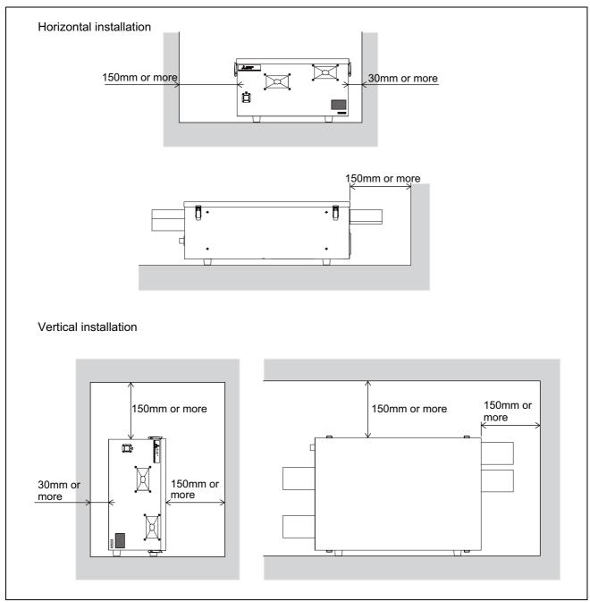
Fig.3-23: Installation dimensions
