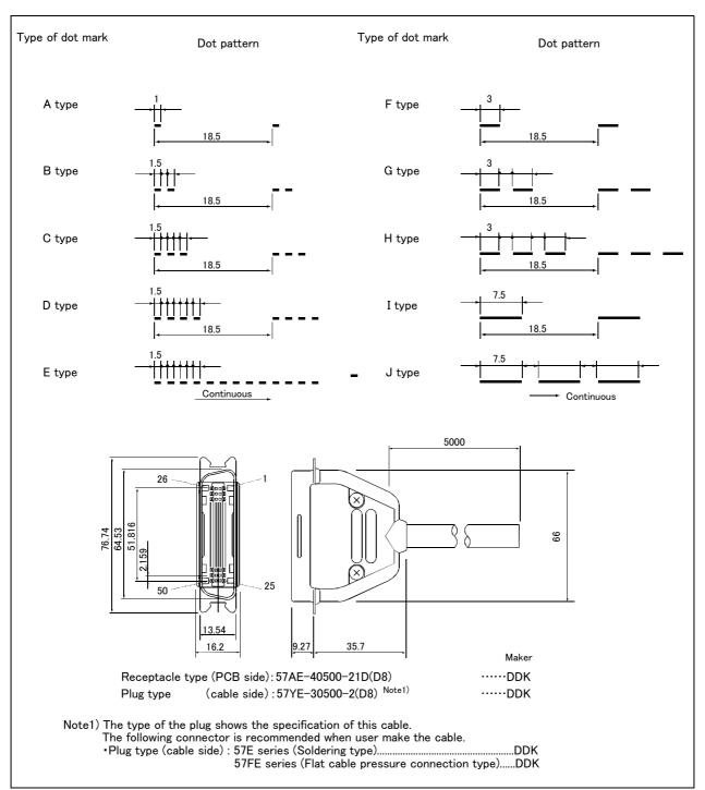
Fig.3-39: Connections and outside dimensions
