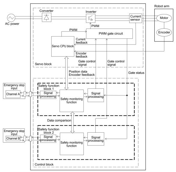
Fig.7-3: Safety block diagram
