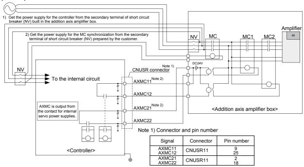
Note 2) This output is opened, if the robot turns off the servo by occurrence of alarm etc. <Electric specification> DC24V/10mA to 100mA
