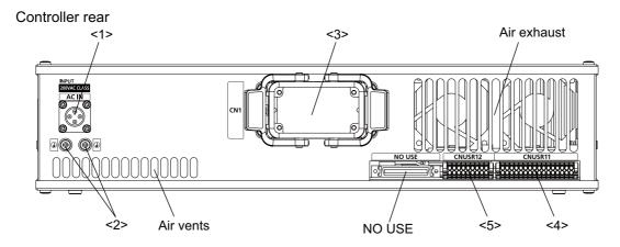
Fig.3-1: Names of controller parts
