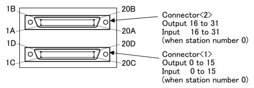
Fig.3-25: Pin layout of connector
