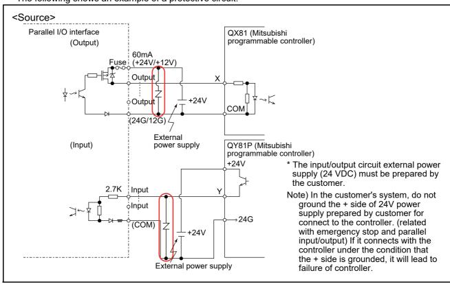
Fig.3-29: Connection with a Mitsubishi PLC (Example of source type) for use of a protective circuit
