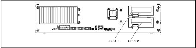
Fig.3-24: Parallel I/O interface installation position
