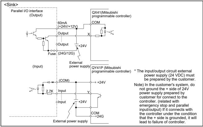
Fig.3-26: Connection with a Mitsubishi PLC (Example of sink type)
