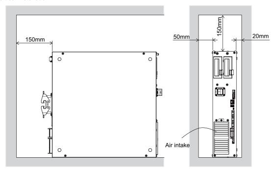
Fig.3-3: Installation dimensions
