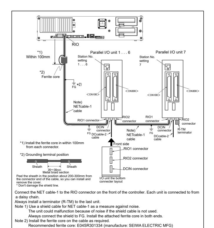
Fig.3-33: Connection method of expansion parallel I/O unit
