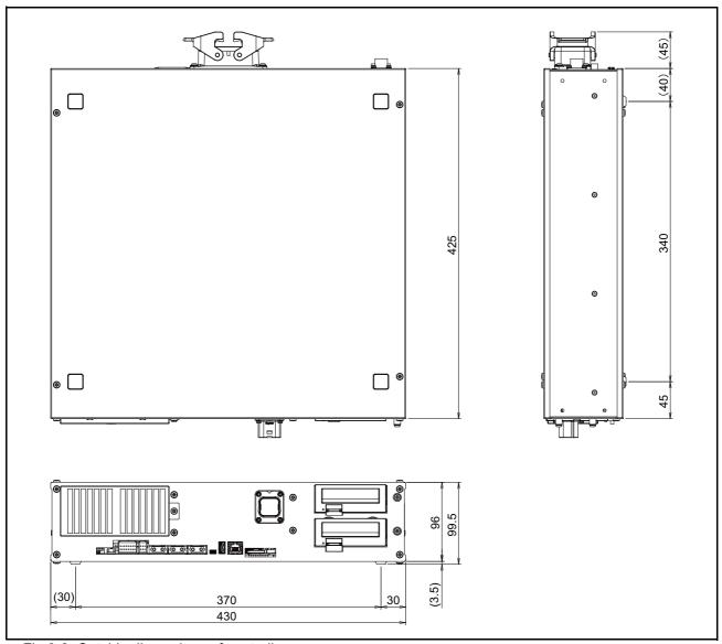
Fig.3-2: Outside dimensions of controller
