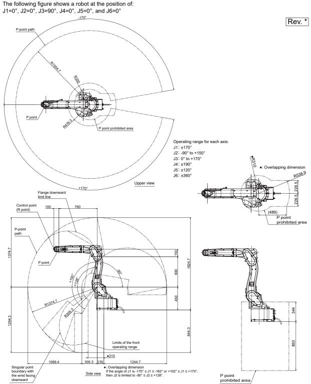
\*1) P point prohibited area: P point cannot enter the area shown in the diagram. However, parameter "MELTEXS" can be used to disable the P point prohibited area. The prohibited area is enabled from the factory.
