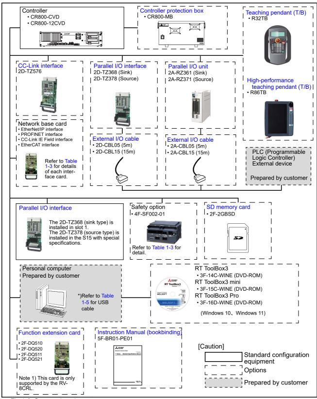
Fig.1-2: Structural equipment
