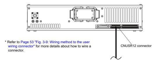
Note) In the customer's system, do not ground the + side of 24V power supply prepared by customer for connect to the controller. (related with emergency stop and parallel input/output) If it connects with the controller under the condition that the + side is grounded, it will lead to failure of controller.
