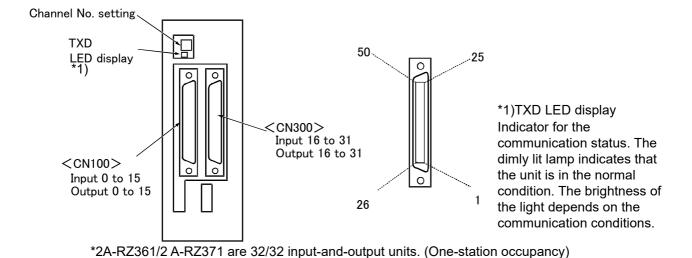
Fig.3-34: Pin arrangement of the parallel I/O unit
