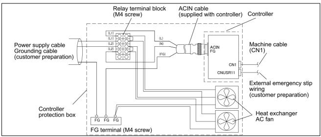
Fig.3-22: Wiring system diagram
