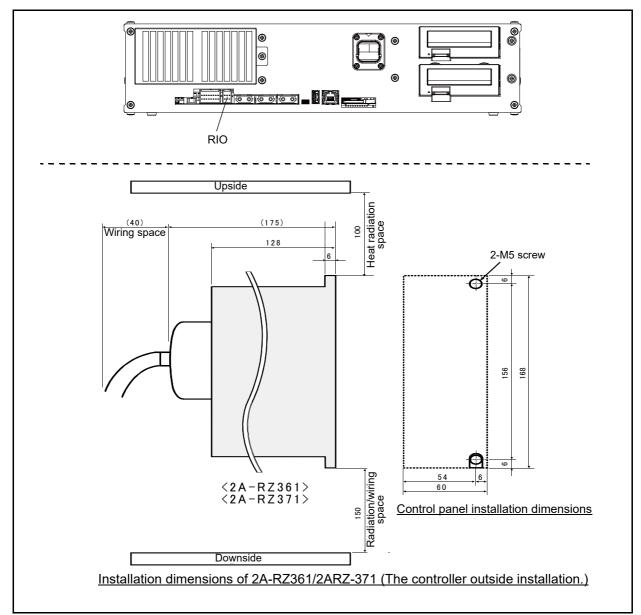
Fig.3-32: Installing the parallel I/O unit
