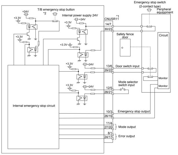
\*1) The CNUSR11 connector is a two-level terminal block, indicating that there are two circuits (channels). Two terminals (cable insertion holes) need to be used for one circuit.
