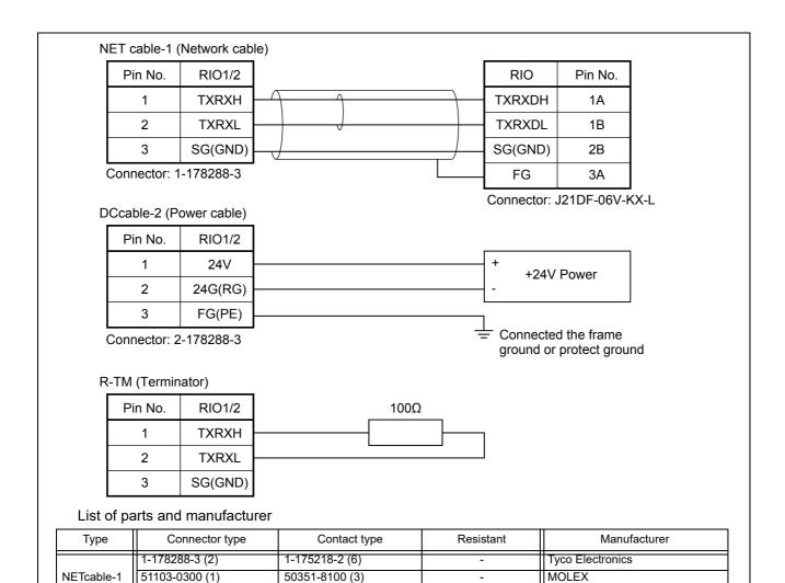
Note 1) The 24V power supply is prepared by customer (The power consumption is approx. 0.3A.)
