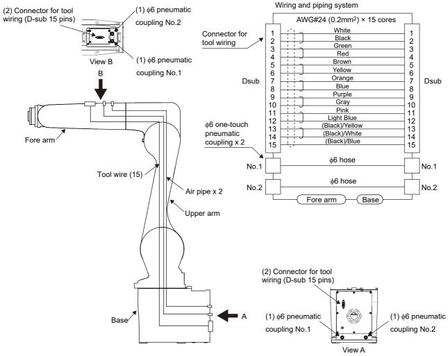
Fig.2-8: Wiring and piping for hand
