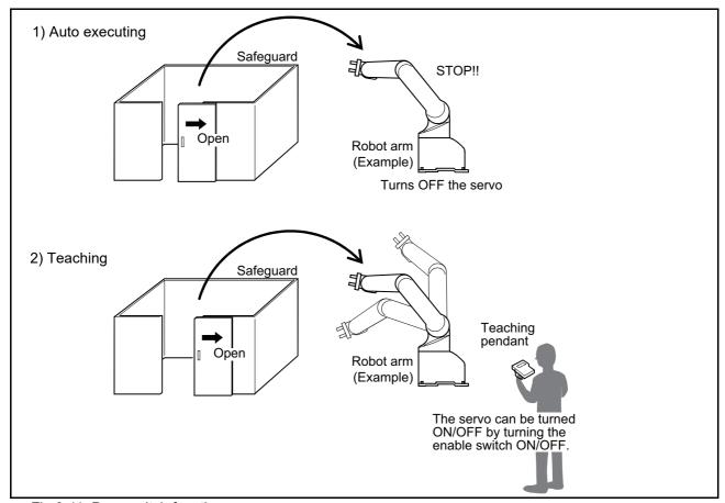
Fig.3-11: Door switch function
