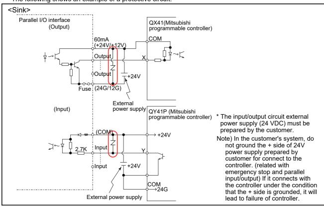
Fig.3-27: Connection with a Mitsubishi PLC (Example of sink type) for use of a protective circuit
