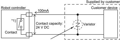
Use noise prevention methods that are specific to the devices being used and the environment they are being used in.
