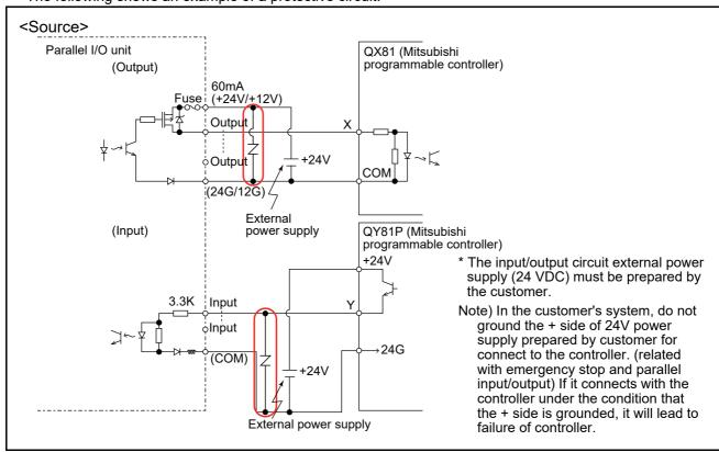
Fig.3-38: Connection with a Mitsubishi PLC (Example of source type) for use of a protective circuit
