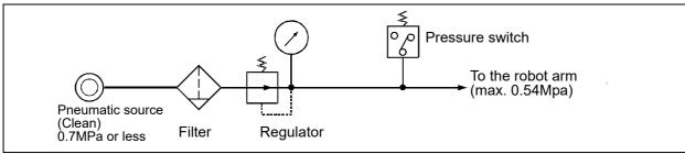
Fig.2-10: Air supply circuit example for the hand
