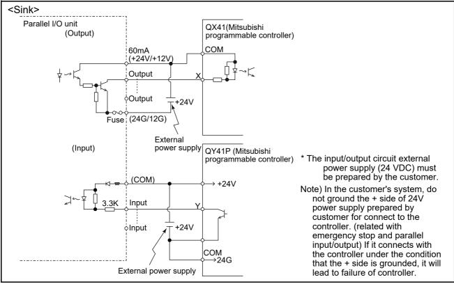
Fig.3-35: Connection with a Mitsubishi PLC (Example of sink type)
