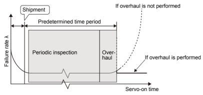
Fig.2-12: Periodic inspection/overhaul periods
