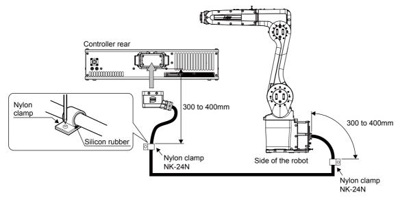
Fig.2-11: Fixing the flexible cable
