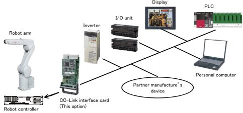
Fig.3-40: Example of CC-Link Product Configuration
