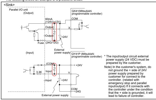
Fig.3-36: Connection with a Mitsubishi PLC (Example of sink type) for use of a protective circuit
