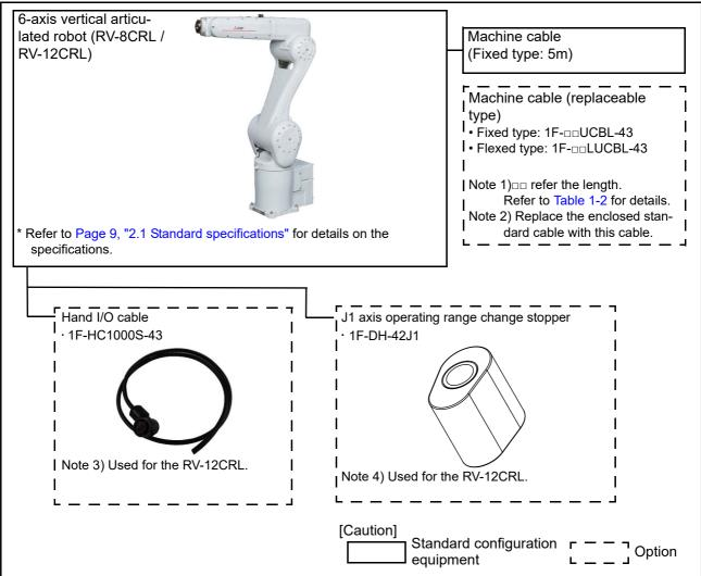
Fig.1-1: Structural equipment
