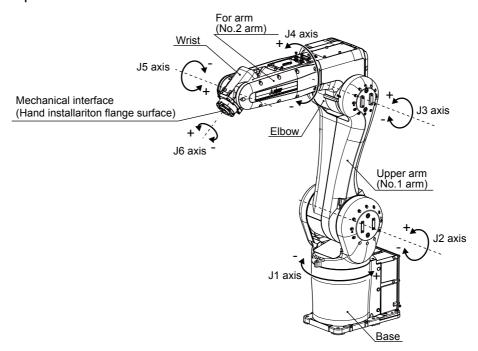
Fig.2-3: Names of each part of the robot
