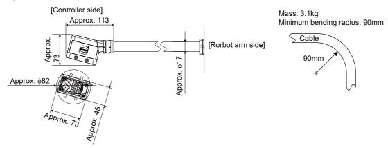
Note) When using machine cables (replaceable type), refer to Page 28, "(1) Machine cable (replaceable): Fixed type" for the cable diameter.
