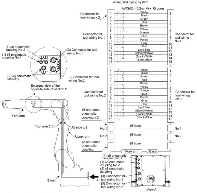
Fig.2-9: Wiring and piping for hand
