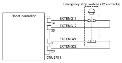
Fig.7-2: How to wire emergency stop lines
