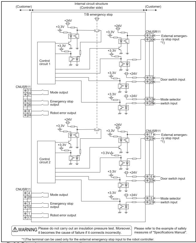
Fig.3-8: External emergency stop connection
