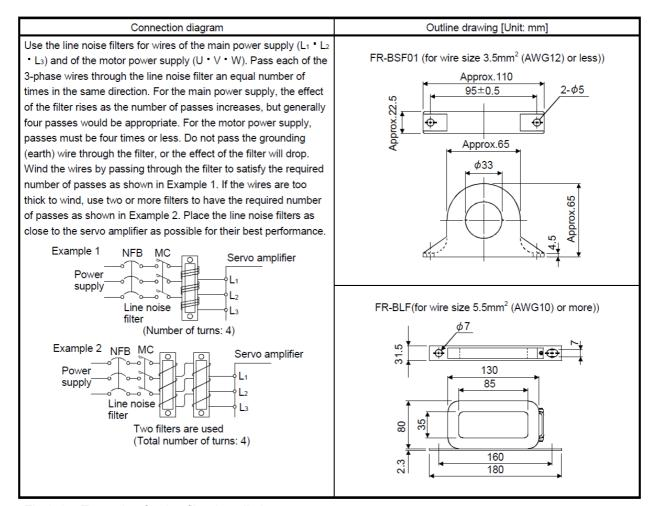
Fig.3-15: Example of noise filter installation
