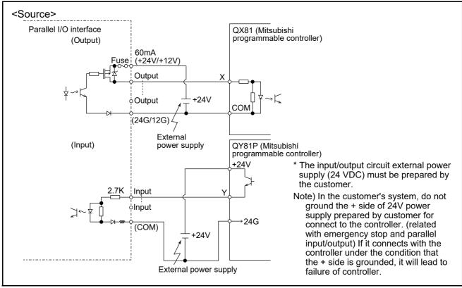
Fig.3-28: Connection with a Mitsubishi PLC (Example of source type)
