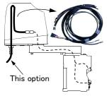
This set, consisting of air hoses and cables, is for feeding air hoses and hand input signal cables from the No. 2 arm through to the shaft tip.
