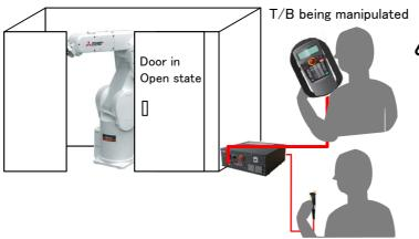
Enabling device being manipulated
