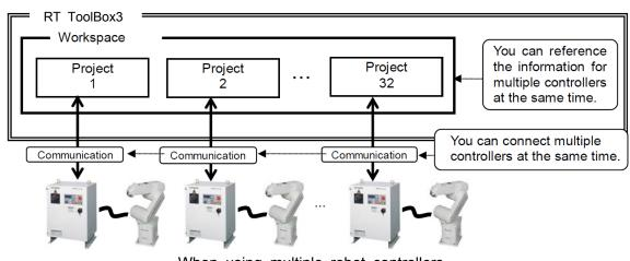
When using multiple robot controllers
