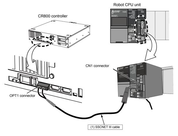
Cable connection between robot CPU unit and CR800 controller
