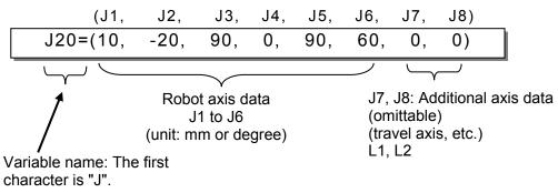
Example) J21=(0, 10, 90, 10, 90, 90, 0, 200) ·······[6-axis robot + additional axis] J22=(10, 90, 30, 10) ······[4-axis robot] J23=(10, 90, 30, 10, , , 0, 200) ······[4-axis robot + additional axis]
