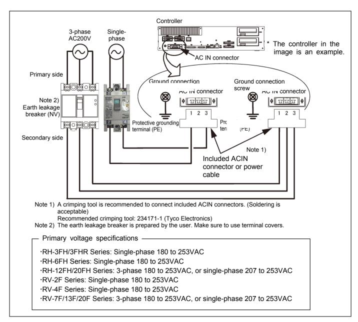
The earth leakage breaker, primary power supply connection cable and earth cable are to be prepared by the customer.
