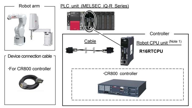
Note 1) The same type of robot CPU module is used for both robot arm types. The CPU is mounted on the PLC unit (base board, power module, PLC CPU required) prepared by the user.
