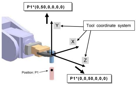
Using the robot tool coordinate, you can operate the robot along the hand surface direction. This enables the adjustment of the hand posture for the target workpiece and easy change of the posture of the held workpiece.
