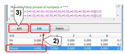
4) To create a new position variable or change the variable name, input a variable name in the Edit Position data window.
