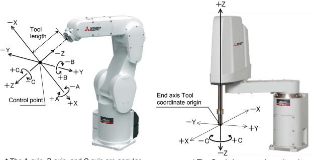
\* The A axis, B axis, and C axis are angular units and change the direction of the flange surface while maintaining the control point position. \* The C axis is an angular unit and changes its direction by changing the end axis.
