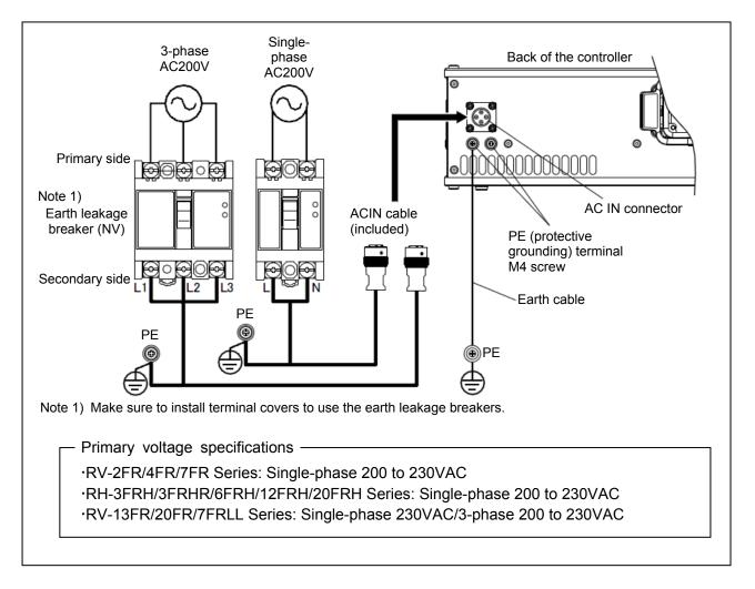
The earth leakage breaker, primary power supply connection cable and earth cable are to be prepared by the customer.
