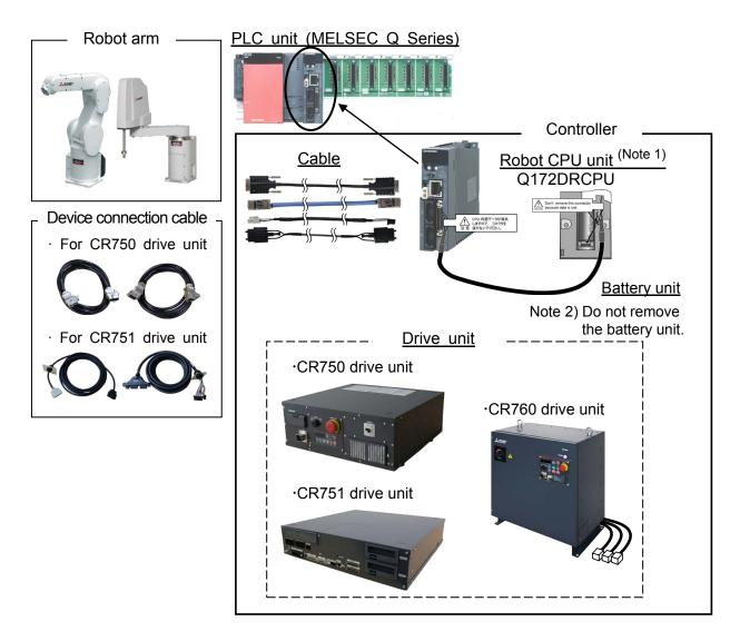
Note 1) The same type of robot CPU module is used for both robot arm types. The CPU is mounted on the PLC unit (base board, power module, PLC CPU required) prepared by the user.
