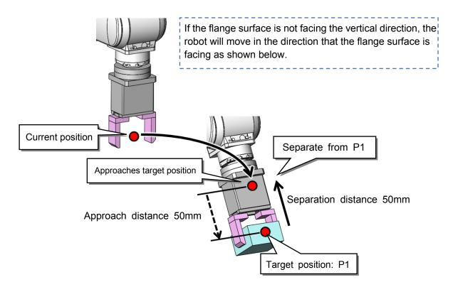
Position data addition/subtraction The addition/subtraction is made with mutual data elements.
