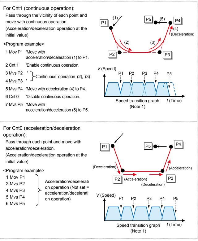
Note 1) "Speed transition graph" shown above is an example. Depending on the movement distance and speed, acceleration/deceleration may occur during interpolation connection.
