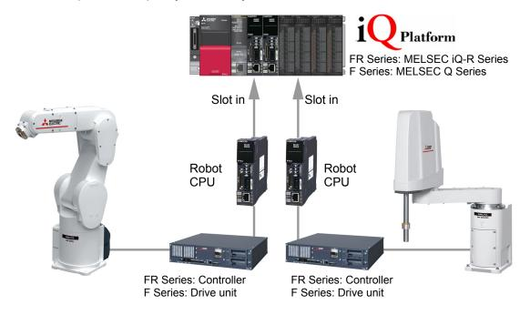
When using an iQ Platform compatible type robot for the first time, a multi-CPU setup is ne cessary.
