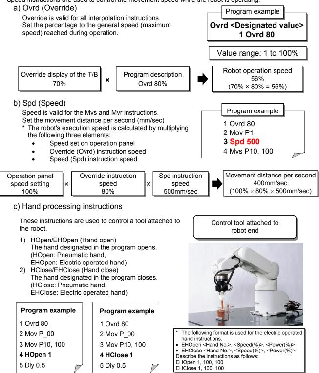
When using the pneumatic hand, the hand numbers 1 to 4 are used for the double solenoid, and numbers 1 to 8 for the signal solenoid. When using the electric operated hand, the hand numbers are 1 to 3.
