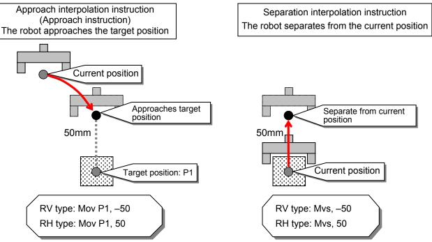
**Note 1)** The approach distance and separation distance are expressed as values in the tool coordinate system's Z axis direction.
