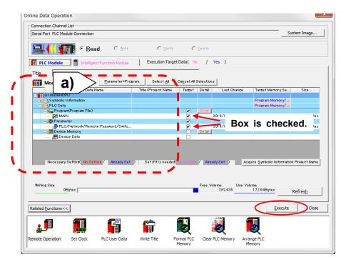
8) The "PC READ" window opens, and data is read from the PLC. When all of the data has been read out, click the "CLOSE" button.
