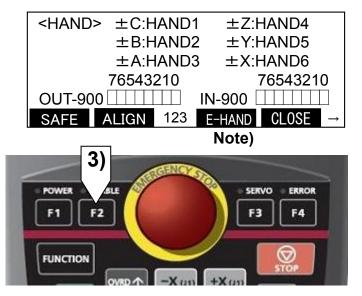
Note) "Electric" appears only when using the electric operated hand. If the function key ([F3] key in this case) corresponding to this is pressed, the <Electric Operated Hand Operation> screen will open.
