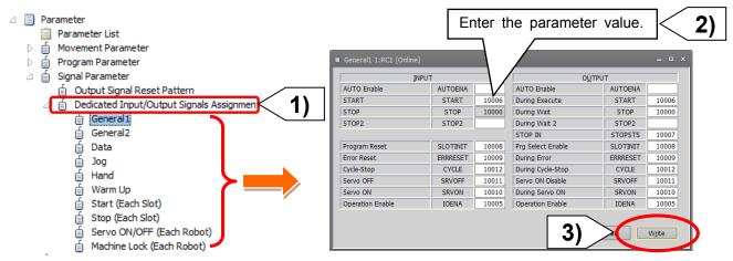
\* After changing the parameters, always turn the controller/drive unit control power OFF and ON. Turning off and on the control power supply of the controller/drive unit enables the changed parameters.
