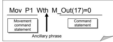
The robot turns off the output number 17 while moving to P1.
