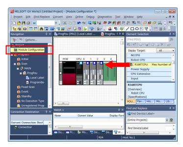
GX Works3 Module Configuration screen example (three robots)
