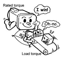
• The load inertia moment should not exceed approximately 10 times of the inertia moment of the motor itself.
