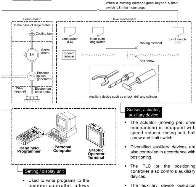
position controller, allows setting and display of the data.
