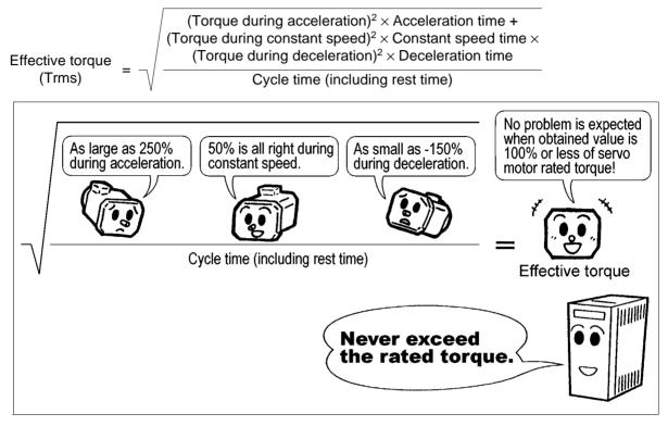
In the effective torque calculation equation, the torque during acceleration, constant speed, deceleration, the cycle time and the machine load are as follows.
