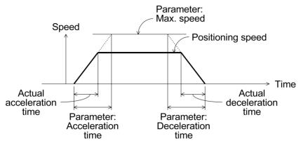
• This operation pattern is effective during return to the zero point, positioning and jog operation.
