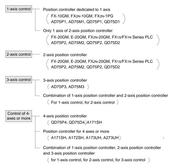
b) Determine the position controller to be used in accordance with the output pulse frequency.
