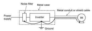
Fig.7.24 Reduction of noise radiated from the inverter
