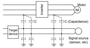
Fig.7.16 Electrostatic induction noise
