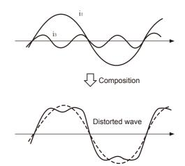
Fig.7.1 Fundamental wave and harmonics
