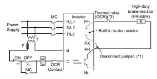
\*1 Since the inverter without built-in brake resistor is not provided with the PX terminal, a jumper is not need to be removed.
