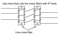
When the thickness of the wire prevents twisting, use at least four filters in series.
