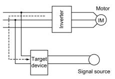
Fig.7.17 Electrical path propagated noise
