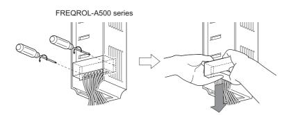
Note 1: The wiring cover of the FREQROL-A500 cannot be installed on the FREQROL-A700. If the FREQROL-A500 has a wiring cover, disconnect the cables from the terminal block instead.
