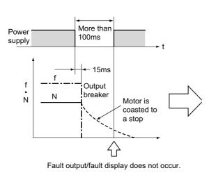
Fig.7.8 Instantaneous power failure over 100ms
