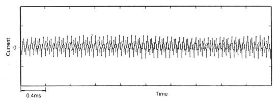
Fig.7.27 Example of earth (ground) cable current of the motor when driven by inverter (Inverter: 200V class 0.75K, Motor: SF-JR 0.75kW 4P)
