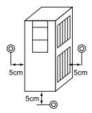
Fig.7.28 Measuring surrounding air temperature
