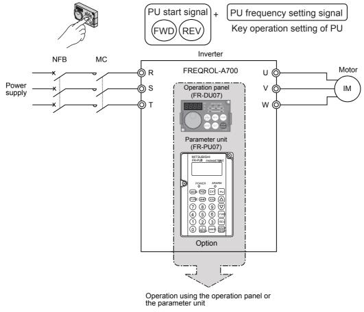
Figure 2.4 PU operation
