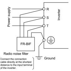
Fig.7.18 Installation of the radio noise filter FR-BIF
