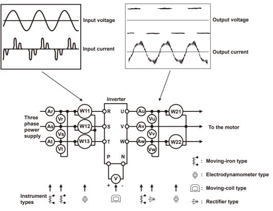
**Examples of Measuring Points and Instruments**
