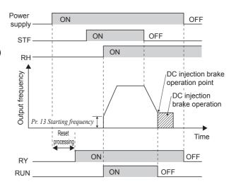
3) Checking the inverter operating status by the start signal input to the inverter and inverter running signal.
