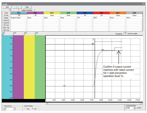
2) Check that the stop by the stall prevention (E.OLT display) occurs at the output current that is lower than the normal value.
