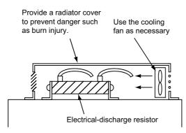
Caution: The surface of the discharge resistor may reach up to about 300°C. Therefore, be careful of the material of the installation side and the location when using two or more discharge resistors.
