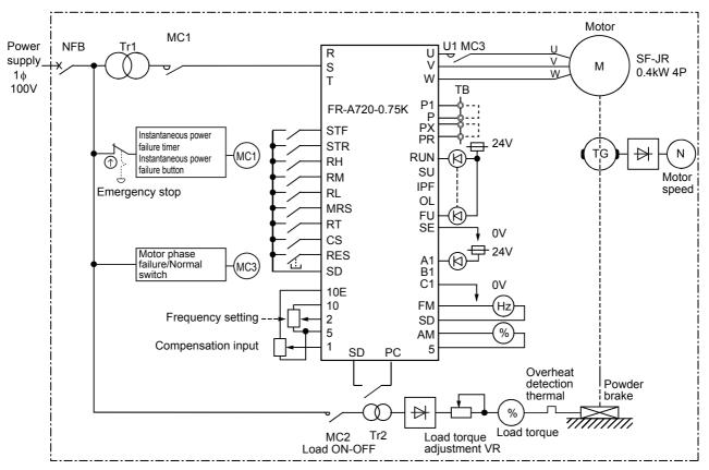
Figure 2.1 Expanded view of the inverter demonstration machine
