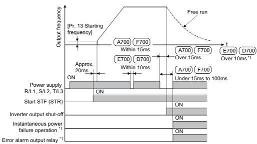
The time chart when instantaneous power failure occurs to the inverter
