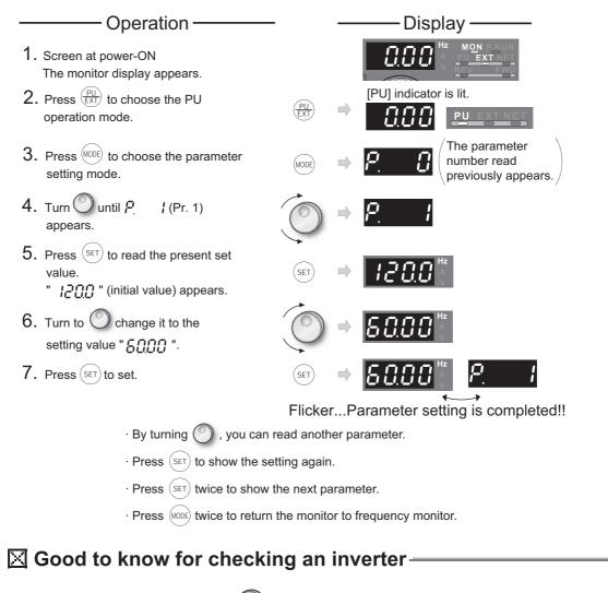
Press the setting dial M ( ) to display the current set frequency.
