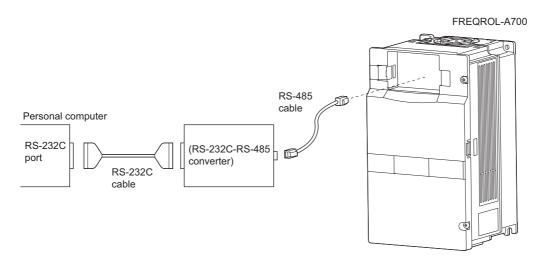
(4) Turn ON the computer and start up the FR Configurator (FR-SW3-SETUP). Click [Parameter List] in [Functions].
