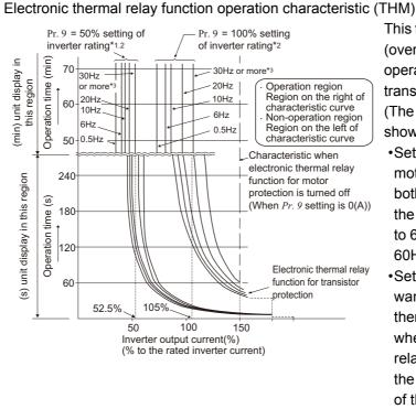
This function detects the overload (overheat) of the motor, stops the operation of the inverter's output transistor, and trips.
