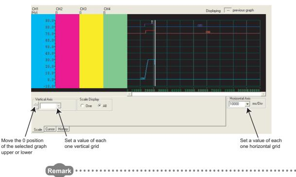
In this example, "Position [%]" is set to "90%". The fault occurrence during the 90% of the sampling time after clicking <u>start</u> (during Pre-Trigger state) is ignored, and sampling is not started.
