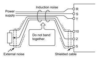
Fig.7.38 Connection example of frequency setting input terminal
