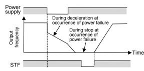
Original operation continuation at instantaneous power failure function When an instantaneous power failure is detected, the operation continues by using regenerative energy which occurs when decelerating. and accelerates until reaching command frequency after restart.
