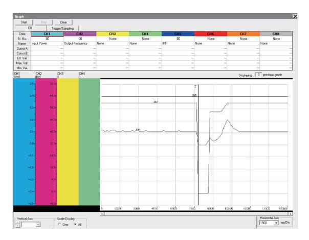
(3) Setting Decelerate the motor to a stop at instantaneous power failure function (Pr.261 to Pr.266, Pr.294)
