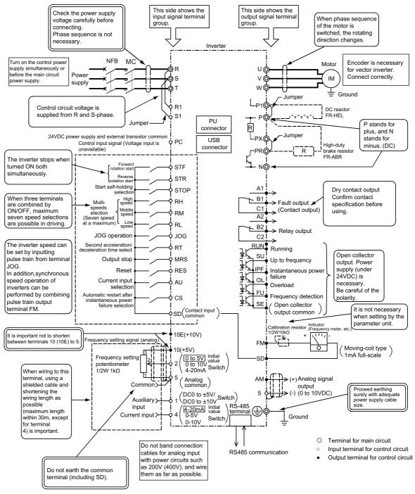
Fig.7.35 Terminal connection
