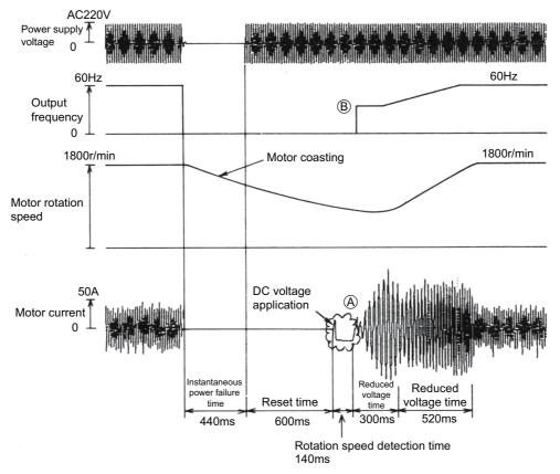
Fig.7.9 Example of instantaneous power failure restart operation
