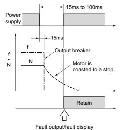
Fig.7.6 Instantaneous power failure of 15ms or lower
