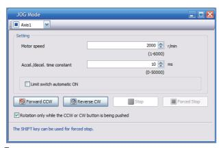
After the test operation is complete, set [Pr. PC05.1 Test operation selection] back to "0" (disabled).
