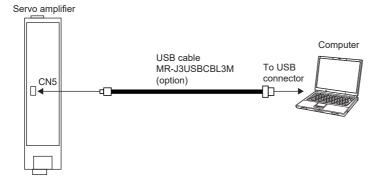
2. Start MR Configurator2 and create a new project. For the connection setting, select USB. Select the servo amplifier model.
