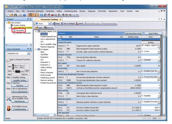
**4.** Select a group of servo parameters in the selection tree of the "Parameter Setting" window to display and configure the settings.
