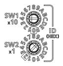
The rotary switches are set to 01h when shipped from the factory.
