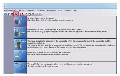
**4.** To operate the servo motor, input the motor speed and acceleration/deceleration time constants, then click "Forward CCW" or "Reverse CW". The servo motor operates only while the button is being clicked. Give a low speed command at first and check the operation status.
