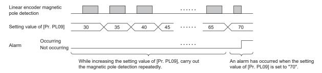
In this example, set the final setting value of [Pr. PL09 Magnetic pole detection voltage level] to 49 (setting value at the alarm occurrence =  $70 \times 0.7$ ).
