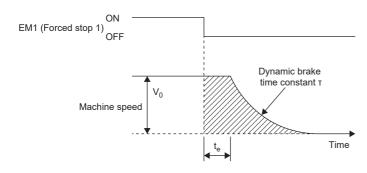
$$L_{max} = \frac{V_0}{60} \cdot \left\{ t_e + \tau \left( 1 + \frac{J_L}{J_M} \right) \right\} \cdots (5.2)$$
