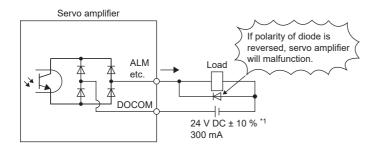
\*1 If the voltage drop (a maximum of 2.6 V) interferes with the relay operation, apply high voltage (a maximum of 26.4 V) from an external source.
