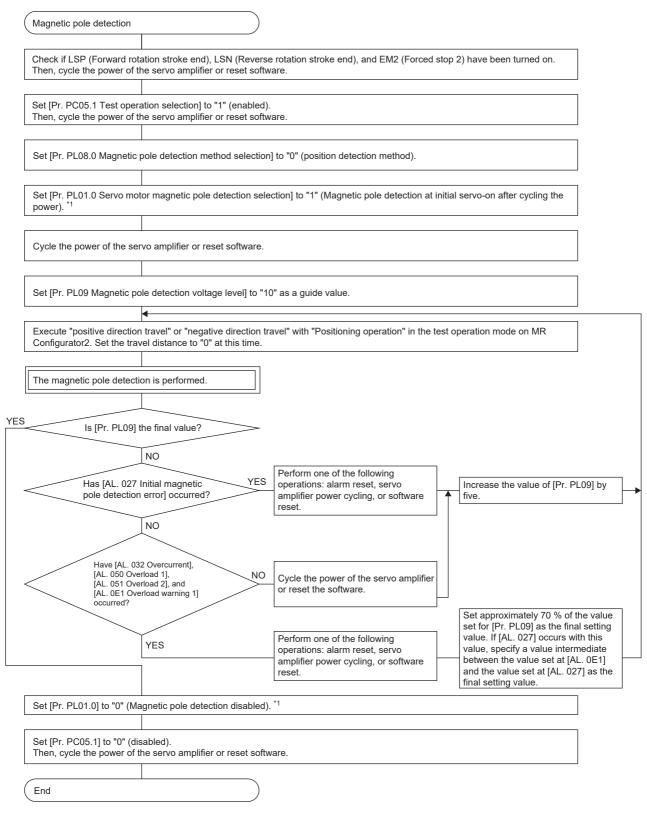
\*1 For the incremental system, the setting of [Pr. PL01] is not required.
