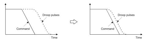
• To suppress vibration: Decrease the value for the dual feedback filter.
