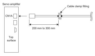
· When using a data line filter
