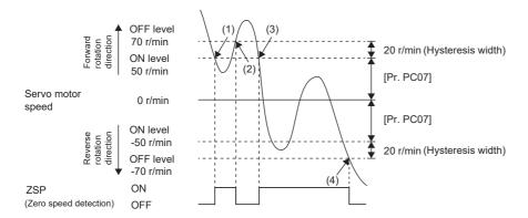
ZSP will turn on when the servo motor speed is reduced to 50 r/min (at (1)), and will turn off when the servo motor is increased to 70 r/min again (at (2)).
