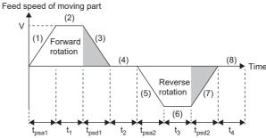
V: Feed speed of moving part [mm/min]
