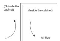
When air flows along the outer wall of the cabinet, effective heat exchange is possible, because the temperature slope inside and outside the cabinet is steeper.
