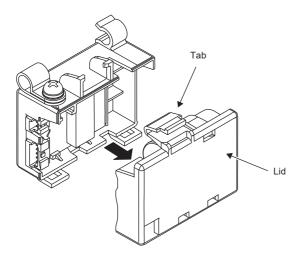
**3.** Pull the battery leads through the hole in the lid, then remove the battery and replace it with a new MR-BAT6V1 battery. Once the battery has been replaced, pull the battery leads through the hole in the lid. Insert the new MR-BAT6V1 battery into the case lid so that the label is visible.
