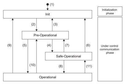
The controller and the servo amplifier perform the following procedure to establish communication (transition to "Operational").
