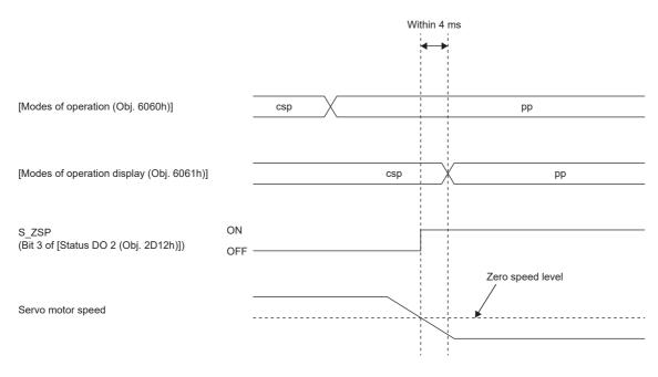
· Control switching for continuous operation to torque control mode (ct)
