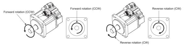
The positive and negative directions of the linear servo motor are as follows.
