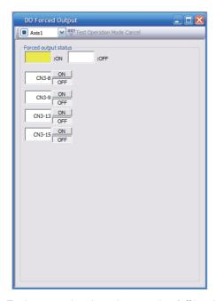
Each output signal can be turned on/off by clicking the ON/OFF button next to its name. After checking, click "Test Operation Mode Cancel" and terminate the output signal (DO) forced output.
