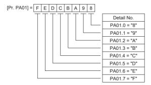
· When setting a servo parameter using a combination of several digits
