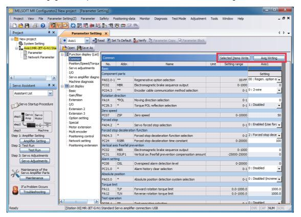
**6.** Abbreviated servo parameters prefixed with \* and servo parameters marked with \*\* are enabled after the power is cycled or a software reset is performed. Click "Software Reset" in MR Configurator2 to perform the software reset.
