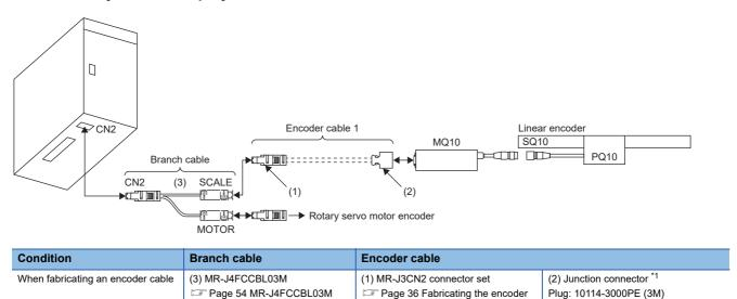
cable used to connect the servo
