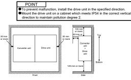
4 Electrical Installation and configuration diagram
