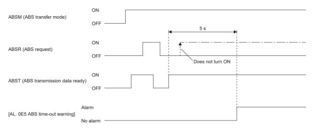
• ABS request on-time time-out check (applied to 32-bit absolute position data in 2-bit units + checksum) If the ABSR is not turned off by the programmable controller within 5 s after ABST is turned off, this will be treated as a transmission error and [AL. 0E5] occurs.
