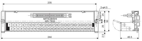
Terminal screw: M3.5 Applicable wire: 2 mm<sup>2</sup> Crimp terminal width: 7.2 mm or less
