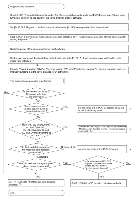
\*1 For the incremental system, the setting of [Pr. PL01] is not required.
