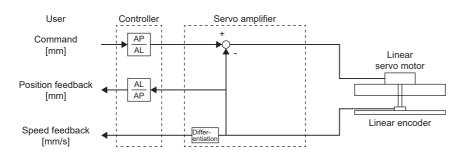
Calculate the number of linear encoder pulses (AP) and travel distance (AL) with the following condition.
