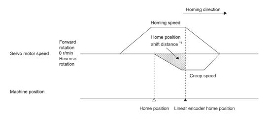
\*1 Home position shift distance can be changed with [Pr. PT07]. When the servo motor returns at the stroke end
