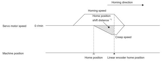
\*1 Home position shift distance can be changed with [Pr. PT07 Home position shift distance]. When the stroke end is detected
