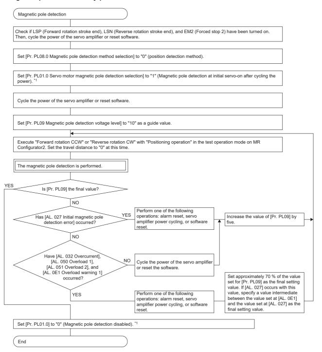
\*1 For the incremental system, the setting of [Pr. PL01] is not required.
