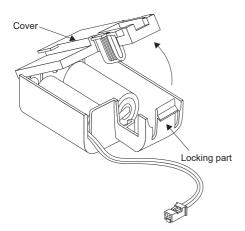
2. Replace the battery with a new MR-BAT6V1 battery.
