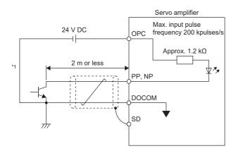
\*1 A photocoupler is used as the pulse train input interface. Therefore, this circuit may not operate properly due to reduction in current if a resistor is connected to the pulse train signal line.
