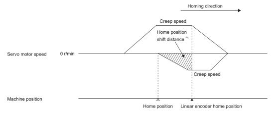
\*1 Home position shift distance can be changed with [Pr. PT07 Home position shift distance]. When the servo motor returns at the stroke end
