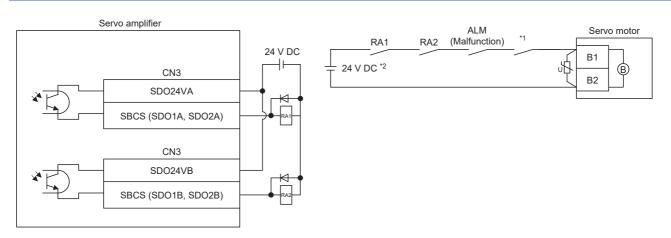
\*1 The circuit should be shut off in conjunction with the emergency stop switch.
