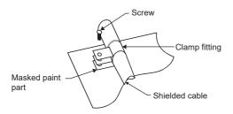
Ground both ends of the cable of the CN3 safety signal with the cable clamp. The shield length from the servo amplifier to the cable clamp should be within 30 cm.
