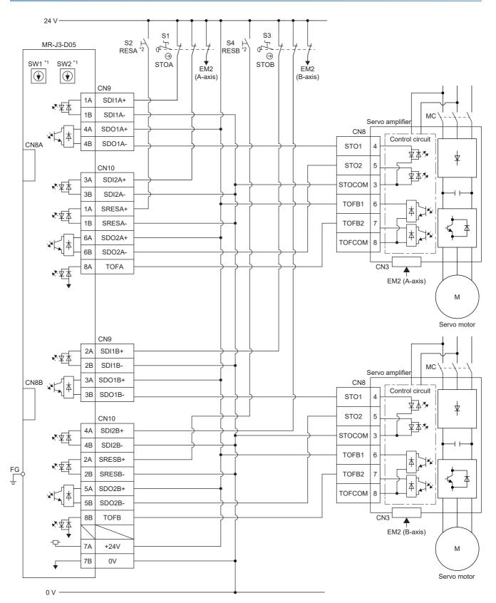
\*1 Set a delay time for STO output with SW1 and SW2. These switches are located in a recessed area in the MR-J3-D05 to prevent accidental setting changes.
