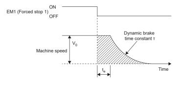
$$L_{max} = \frac{V_0}{60} \cdot \left\{ t_e + \tau \left( 1 + \frac{J_L}{J_M} \right) \right\} \cdots (10.2)$$
