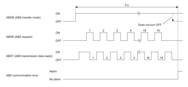
3. After the ABS request signal turns on, check the time it takes to turn off (ABS transfer time).
