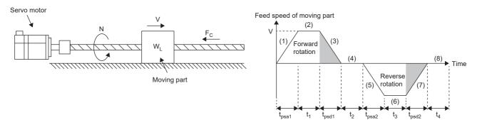
V: Feed speed of moving part [mm/min]
