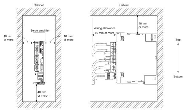
\*1 For the MR-J5-500\_4\_ and MR-J5-700\_4\_, leave a clearance of at least 70 mm between the bottom of the servo amplifier and the cabinet. When using a shield clamp attachment, refer to the following.
