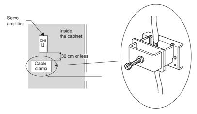
For the grounding of the shield of the I/O signal cable, SCC 15-F (Phoenix Contact) can be used. Refer to the following for details.
