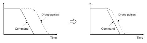
· To suppress vibration: Decrease the value for the dual feedback filter.
