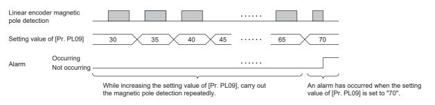
In this example, set the final setting value of [Pr. PL09] to 49 (setting value at the alarm occurrence = 70 × 0.7).
