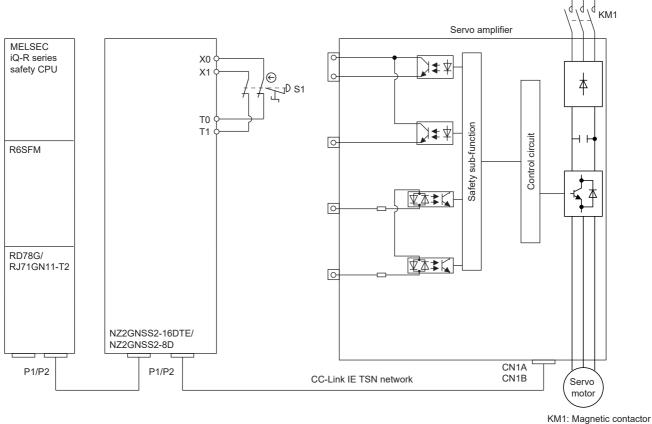
KM1: Magnetic contactor S1: Safety switch
