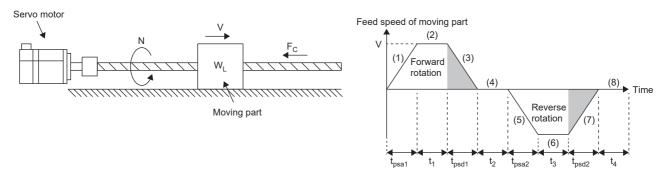
V: Feed speed of moving part [mm/min]
