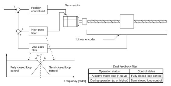
\*1 Set "ω" (dual feedback filter band) with [Pr. PE08 Fully closed loop dual feedback filter].
