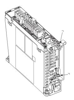
\*1 The recommended screw tightening torque is  $1.5 \pm 0.1$  N•m.
