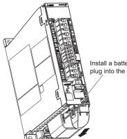
Install a battery, and insert the plug into the CN4 connector.
