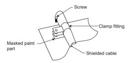
Ground both ends of the CN8 cable with the cable clamp. The shield length from the servo amplifier to the cable clamp should be within 30 cm.
