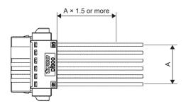
• Prevent the wire from being pulled excessively after the connecter is inserted in the servo amplifier.
