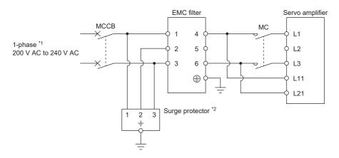
\*1 Connect the power supply to L1 and L3. Leave L2 open.
