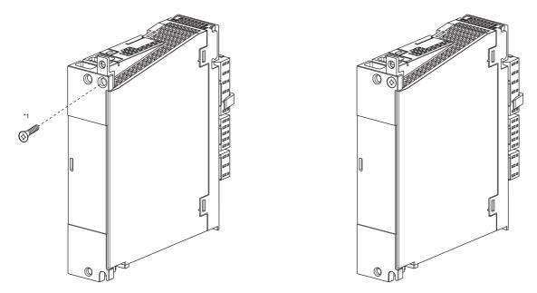
\*1 Use one of the flat head screws included with the attachment. (Tightening torque: 1.2 [N•m])
