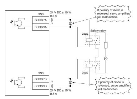
\*1 Incorrect polarity of the power supply causes malfunction of the safety relay.
