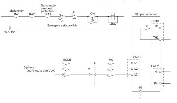
\*1 When connecting a linear servo motor that has a thermal protector, add a contact that interlocks with the thermal protector output of the linear servo motor.
