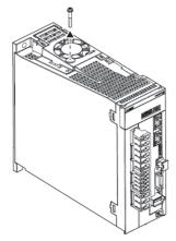
**2.** Pull up the cover of the fan unit using a precision screwdriver.
