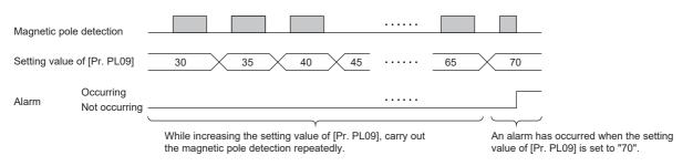
In this example, set the final setting value of [Pr. PL09] to 49 (setting value at the alarm occurrence = 70 × 0.7).
