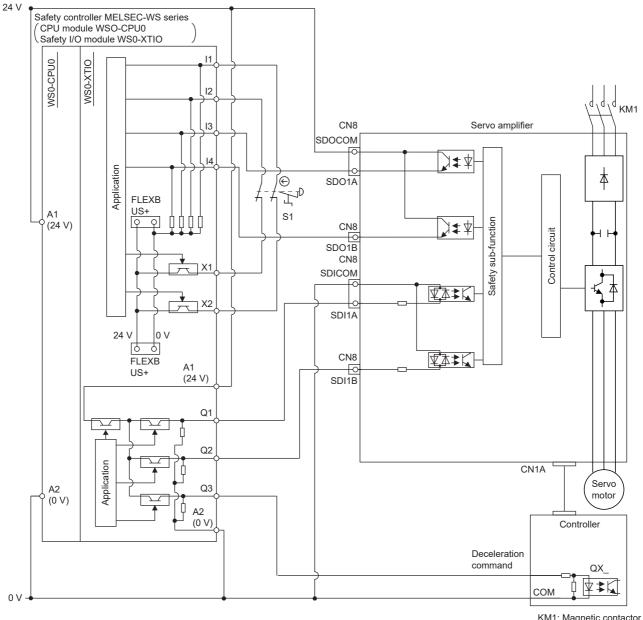
KM1: Magnetic contactor S1: Safety switch
