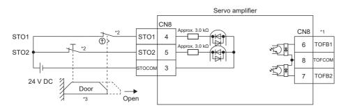
The safety level depends on the setting values of [Pr. PF18 STO diagnosis error detection time] and [Pr. PSD18\_Permissible time for mismatches DI1] and whether STO input diagnosis by TOFB output is performed or not. For details, refer to [Pr. PF18] and [Pr. PSD18] in the following manuals.
