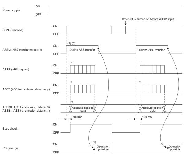
After the absolute position data is transmitted, RD turns on by ABSM-off. When RD is on, ABSM-on is not received. (1) Even if SON is turned on before ABSM is turned on, the base circuit is not turned on until ABSM is turned on. If an alarm occurs, ABSM transfer is not received. If a warning occurs, ABSM transfer can be received. (2) If ABSM is turned off during the ABSM transfer mode, the ABS transfer mode is interrupted and [AL. 0E5 ABS time-out warning] occurs. (3)
