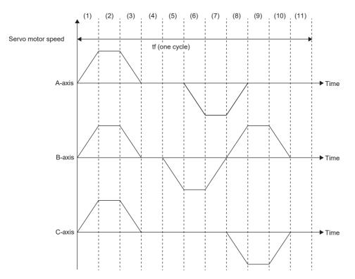
Calculate the energy at each timing in one cycle. Energy is a positive value in power running and a negative value in regeneration. Create a table like the one shown below, and write down the energy during power running/regeneration with signs.
