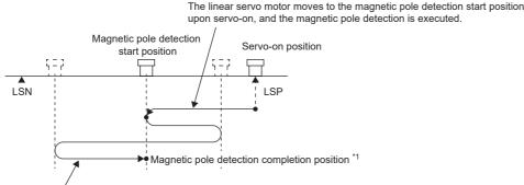
The linear servo motor reciprocates several times and returns to the magnetic pole detection start position to complete the magnetic pole detection, and then changes into the servo-lock status. At this time, there may be a gap, approximately a quarter of the pitch against magnetic pole, from the start position.
