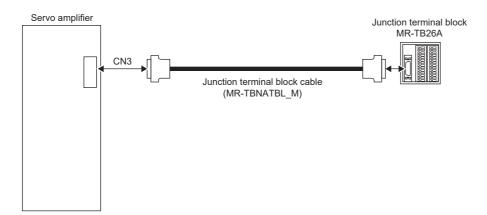
Ground the junction terminal block cable using the S terminal of the junction terminal block.
