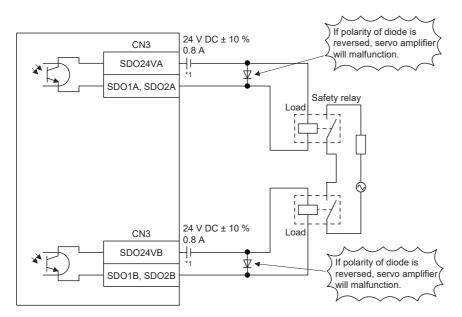
\*1 Incorrect polarity of the power supply causes malfunction of the safety relay.
