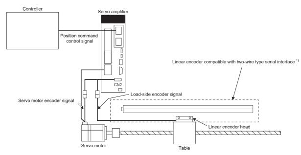
\*1 When using an absolute position linear encoder, an absolute position detection system can be supported. In that case, batteries are unnecessary.
