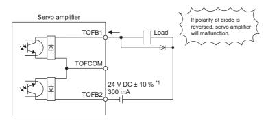
\*1 If the voltage drop (a maximum of 5.2 V) interferes with the relay operation, apply high voltage (a maximum of 26.4 V) from an external source.
