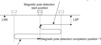
The linear servo motor reciprocates several times and returns to the magnetic pole detection start position to complete the magnetic pole detection, and then changes into the servo-lock status. At this time, there may be a gap, approximately a quarter of the pitch against magnetic pole, from the start position.
