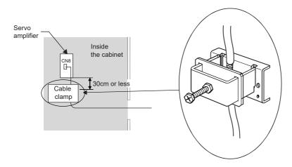
For the MR-J5-500\_4-\_ and MR-J5-700\_4-\_, the shield of the I/O signal cable can be grounded using SCC 15-F (Phoenix Contact). Refer to the following for details.
