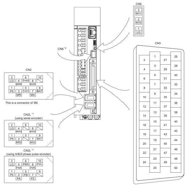
\*1 The MR-J5-\_A\_ servo amplifier does not have the CN2L connector.
