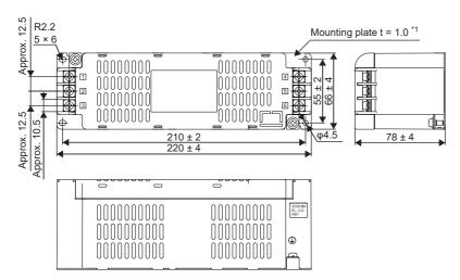
\*1 This applies to HF3030C-SZL. The mounting plate thickness of HF3060C-SZL is 1.2 mm.
