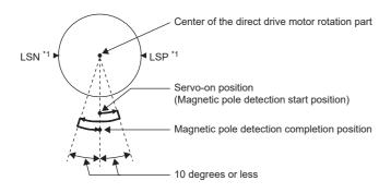
\*1 When LSP (Forward rotation stroke end) or LSN (Reverse rotation stroke end) is turned off during the magnetic pole detection, the magnetic pole detection is carried on to the opposite direction. When both LSP and LSN are off, [AL. 027 Initial magnetic pole detection error] occurs.
