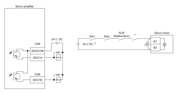
\*1 The circuit should be shut off in conjunction with the emergency stop switch.
