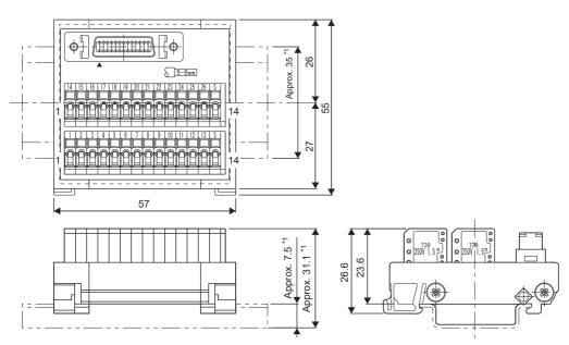
\*1 Values in parentheses are the sizes when installed with a 35 mm DIN rail.
