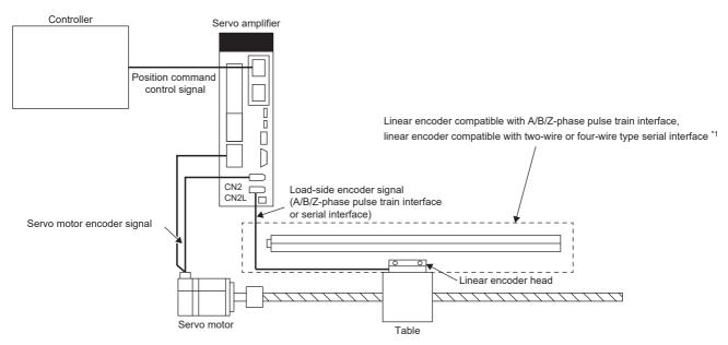
\*1 When using an absolute position linear encoder, an absolute position detection system can be supported. In that case, batteries are unnecessary.
