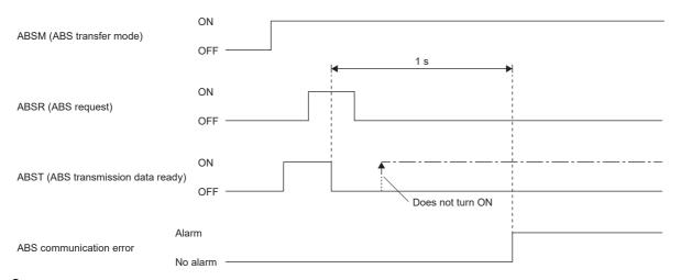
2. After the ABS transfer mode signal turns on, check the time it takes to turn off (ABS transfer time).
