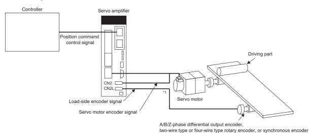
\*1 When an HK-KT servo motor or HK-MT servo motor is used, an absolute position detection system can be supported without using batteries.
