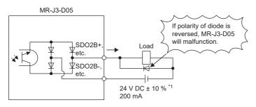
\*1 If the voltage drop (maximum of 2.6 V) interferes with the relay operation, apply high voltage (maximum of 26.4 V) from external source.
