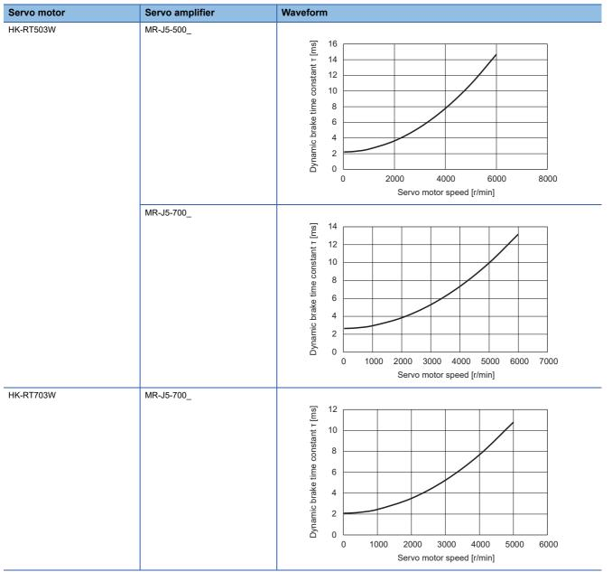
\*1 The dynamic brake time constant is longer than when the HG-RR103 and MR-J4-200\_ are used in combination. To obtain the dynamic brake time constant equivalent to the combination of the HG-RR103 and MR-J4-200\_, use the HK-RT103W and MR-J5-200\_ in combination.
