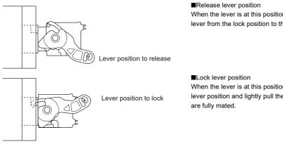
When the lever is at this position, the connector is completely pulled out of the unit. Rotate the lever from the lock position to the release position to lift the terminal block off the unit.
