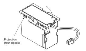
**3.** Press the cover until it is fixed with the projection of the locking part to close the cover.
