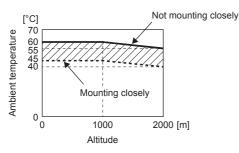
When mounting servo amplifiers close together while using them in environments comparable to those within the diagonal lines in the figure above, use them at an effective load ratio of 75 % or less.
