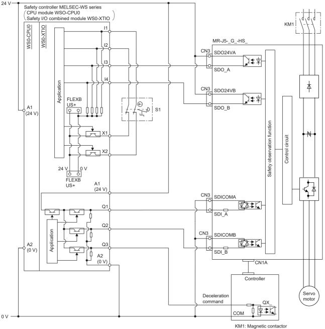
KM1: Magnetic contactor S1: Safety switch
