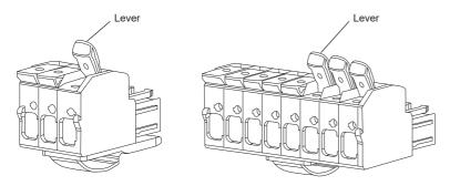
2. Insert a properly stripped wire into the wire insertion hole.
