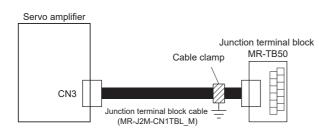
Ground the junction terminal block cable on the junction terminal block side with the supplied cable clamp fitting (AERSBAN-ESET). For the use of the cable clamp fitting, refer to the following.
