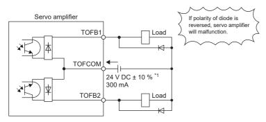
\*1 If the voltage drop (a maximum of 2.6 V) interferes with the relay operation, apply high voltage (a maximum of 26.4 V) from an external source.
