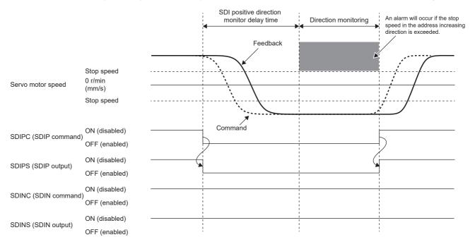
The operation sequence by SDINC (SDIN command) is shown below. The function monitors the address decreasing direction.
