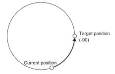
When the current position is 90 and the position data of 270.000 degrees (target position) is specified, the servo motor rotates in CCW direction since the distances in CCW direction and CW direction are the same.
