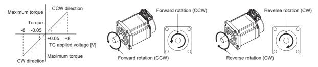
The command value for output torque relative to the voltage varies by approximately 5 % between motors. The torque may vary if the voltage is low (-0.05 V to 0.05 V) and the actual speed is close to the limit value. In such a case, increase the speed limit value.
