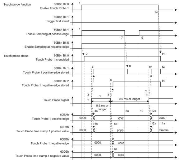
\*1 Change "Touch Probe Signal" so that both the on-time and off-time are 0.5 ms or longer.
