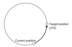
When the position data of -270.000 degrees (target position) is specified, the servo motor rotates in CCW direction.
