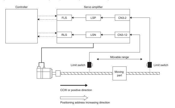
• [Pr. PA14 Travel direction selection] = "1" (CW or the negative direction)
