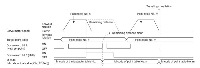
• When "M code update setting" of [Pr. PT83.2\_Positioning function selection 2] is "0" Because the positioning operation is not finished, the M code is not updated from the value before positioning operation even after New set-point.
