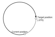
When the position data of -270.000 degrees (target position) is specified, the servo motor rotates in CW direction.
