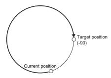
When the position data of -360.000 degrees (target position) is specified, the servo motor rotates in CW direction. (A) When the position data of 360.000 degrees or 0 degree is specified, the servo motor rotates in CCW direction. (B)
