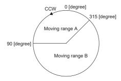
Set servo parameters as follows to specify moving range A.
