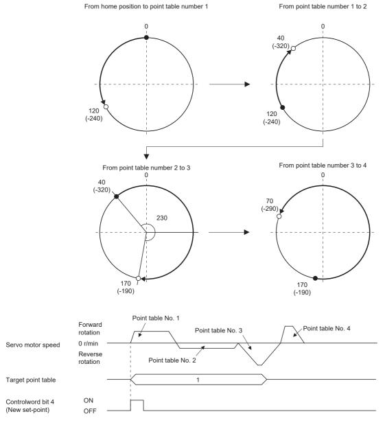
For the operation timing of S\_INP (in-position), S\_CPO (rough match), S\_MEND (traveling completion), [Point actual value (Obj. 2D69h)], [Point demand value (Obj. 2D68h)] and [M code actual value (Obj. 2D6Ah)], refer to "When positioning to the same direction".
