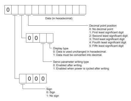
For example, data "00120000270F" means 999.9 (decimal display format) and data "000000003ABC" means 3ABC (hexadecimal display format).
