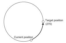
When the position data of -90.000 degrees (target position) is specified, the servo motor rotates in CCW direction.
