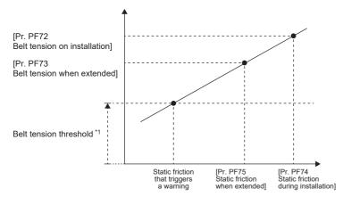
\*1 Belt tension threshold = [Pr. PF76 Belt tension irregular threshold]/100 × [Pr. PF72 Belt tension on installation]
