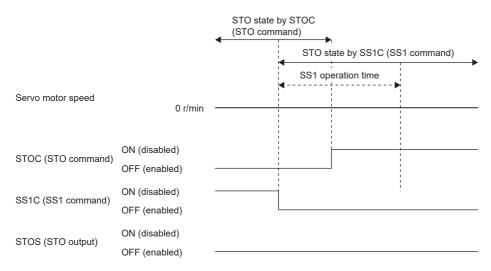
Moreover, if STOC (STO command) is turned off while the SS1 function is being executed, both the deceleration operation of SS1 and time counting are suspended.
