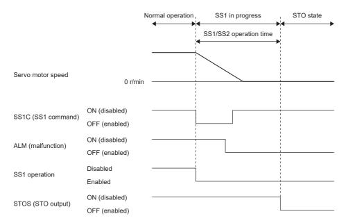
There are two triggers for the SS1 function, namely SS1C (SS1 command) input and ALM (Malfunction), but the only timer that counts the SS1/SS2 deceleration monitor time is the one that was counting from SS1C (SS1 command) that was input first. When SS1C (SS1 command) returns to on, the SS1 function is enabled by ALM (Malfunction), and thus the SS1 function continues the operation.
