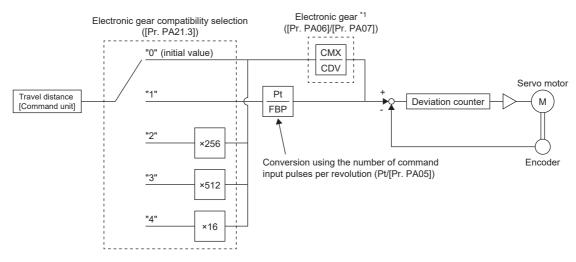
\*1 With CM1 (Electronic gear selection 1) and CM2 (Electronic gear selection 2) of the input device, the setting value of CMX can be selected from [Pr. PA06], [Pr. PC32], [Pr. PC33], or [Pr. PC34].
