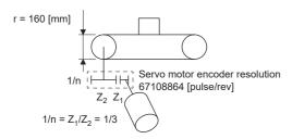
Pulley diameter: r = 160 [mm]Reduction ratio:  $1/n = Z_1/Z_2 = 1/3$
