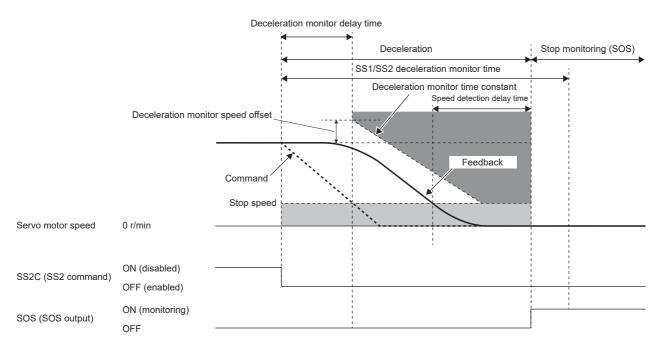
When the servo motor speed is exceeded, the STO function is activated. For the threshold used for judgment, the offset can be set in [Pr. PSA25 SS1/SS2 deceleration monitor speed offset].
