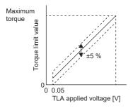
TLA applied voltage vs torque limit value
