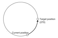
When the position data of -90.000 degrees (target position) is specified, the servo motor rotates in CW direction.
