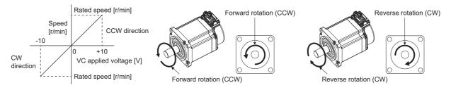
The rotation direction can be selected by using ST1 (Forward rotation start), ST2 (Reverse rotation start), or VC (Analog speed command).
