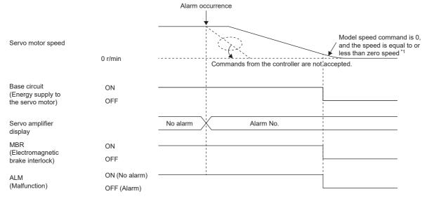
\*1 The model speed command is a speed command generated in the servo amplifier for forced stop deceleration of the servo motor.
