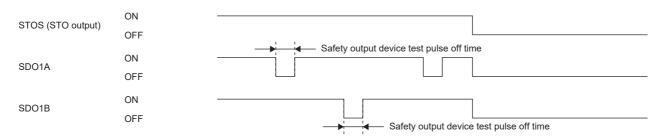
If an error is detected by the test pulse diagnosis, [AL. 556 Output device diagnosis error (safety sub-function)] occurs. Whether or not to perform diagnosis on output devices using test pulses can be selected with [Pr. PSD29 Output device - Test pulse diagnosis execution selection].
