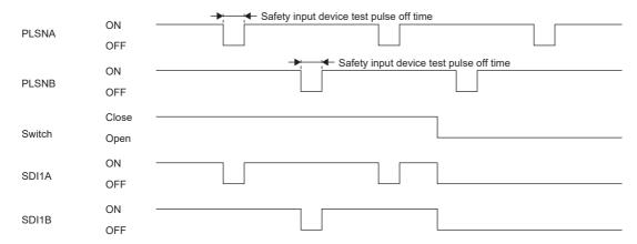
If an error is detected by the test pulse diagnosis, [AL. 553 Input device diagnosis error (safety sub-function)] occurs. Whether to perform diagnosis on input devices using test pulses can be selected with [Pr. PSD24 Safety input device - Test pulse diagnosis execution selection 1].
