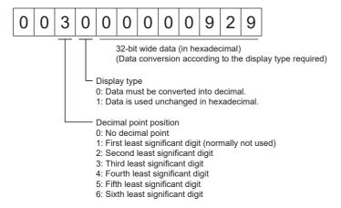
Since the display type is "0" in this case, convert the hexadecimal data into decimal.
