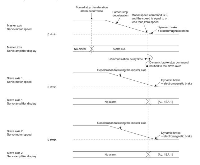
When the slave axes stop the servo motors with the forced stop deceleration due to an alarm detection or other reason, a deceleration request is notified to the master axis. The master axis that has received a deceleration stop request starts forced stop deceleration. When the master axis is in the process of forced stop deceleration, the slave axes decelerate the servo motors in accordance with the torque command and speed limit command from the master axis.
