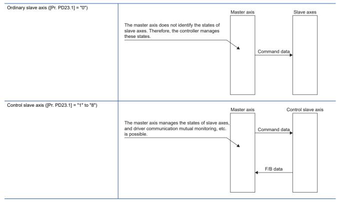
To set a control slave axis, set [Pr. PD23.1 Driver communication setting - Slave - Master axis 1 - Control slave axis No. setting] to any of "1" to "8". If [Pr. PD23.1] of a slave axis is set to "0", the slave axis does not transmit feedback data. Up to eight slave axes can be set as control slave axes per master axis.
