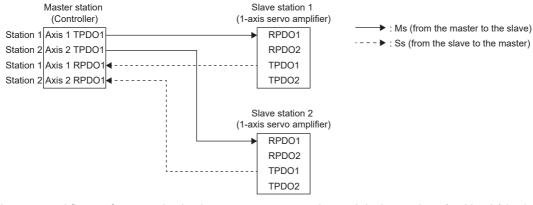
A conceptual figure of communication between a master station and device stations (multi-axis) is shown below.
