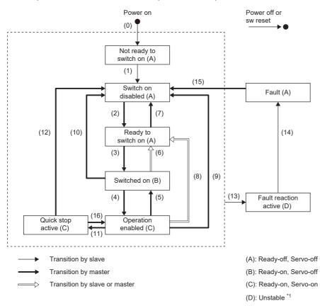
\*1 In the controller that displays the servo-on status by referring to the PDS status, the servo-on status on the controller may differ from the actual servo-on status.
