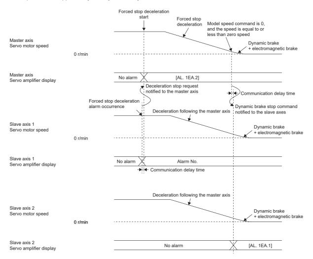
When the slave axes stop the servo motors using the dynamic brakes due to an alarm detection or other reason, the dynamic brakes are activated to stop the servo motors.
