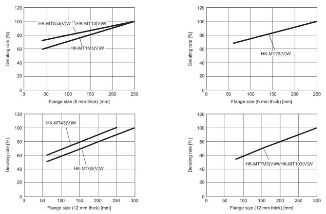
\*1 For the HK-MT053W\_J\_ (with an oil seal), use it at a derating rate of 80 %. When applying the derating in the conditions above, calculate the multiplication of the derating rate of 80 % with an oil seal and the derating rate of each condition, and use the servo motor at the calculated derating rate or lower.
