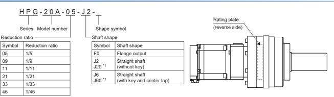
\*1 Only for the gear reducer model 11B
