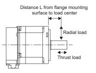
In case where the load position changes, calculate the permissible radial load from the distance measured from the flange mounting surface to the center of the load, and make the load equal to or less than the permissible radial load, referring to the graph shown in the following.
