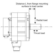
In case where the load position changes, calculate the permissible radial load from the distance measured from the flange mounting surface to the center of the load, and make the load equal to or less than the permissible radial load, referring to the graph shown in the following.
