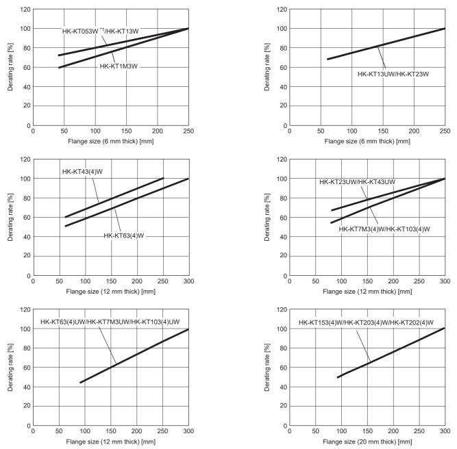
\*1 For the HK-KT053W\_J\_ (with an oil seal), use it at a derating rate of 80 %. When applying the derating in the conditions above, calculate the multiplication of the derating rate of 80 % with an oil seal and the derating rate of each condition, and use the servo motor at the calculated derating rate or lower.
