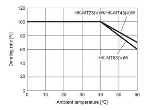
\*1 For the HK-MT053W\_J\_ (with an oil seal), use it at a derating rate of 80 %. When applying the derating in the conditions above, calculate the multiplication of the derating rate of 80 % with an oil seal and the derating rate of each condition, and use the servo motor at the calculated derating rate or lower.
