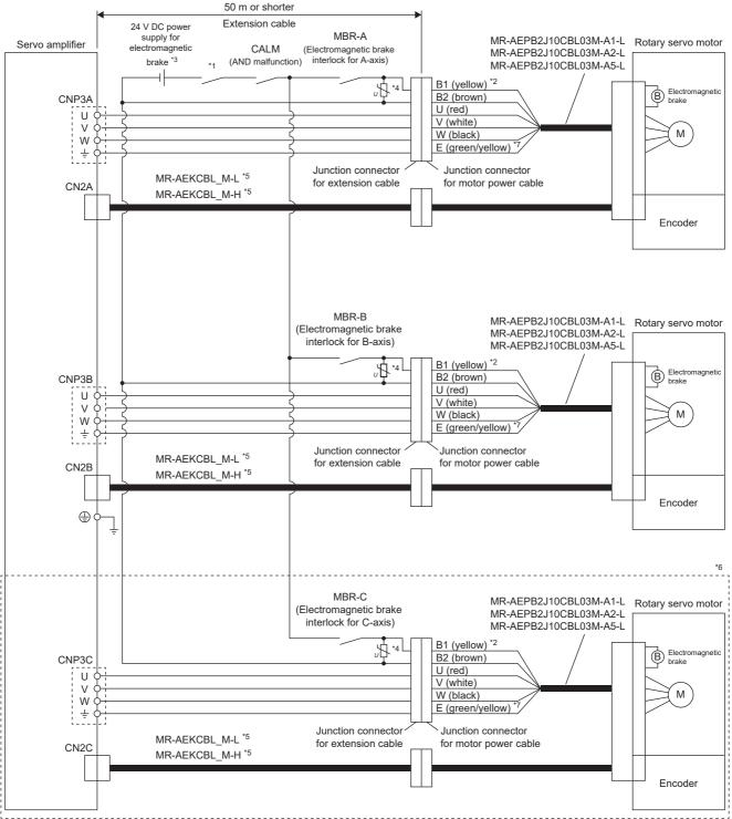
\*1 Configure a circuit which interlocks with an emergency stop switch to shut off.
