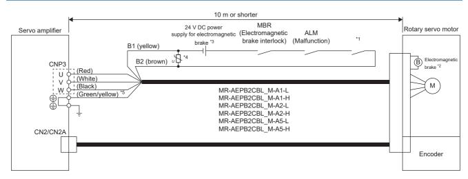
\*1 Configure a circuit which interlocks with an emergency stop switch to shut off.
