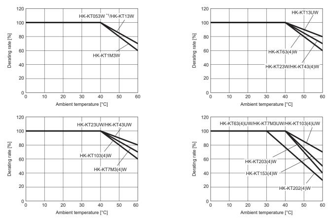
\*1 For the HK-KT053W\_J\_ (with an oil seal), use it at a derating rate of 80 %. When applying the derating in the conditions above, calculate the multiplication of the derating rate of 80 % with an oil seal and the derating rate of each condition, and use the servo motor at the calculated derating rate or lower.
