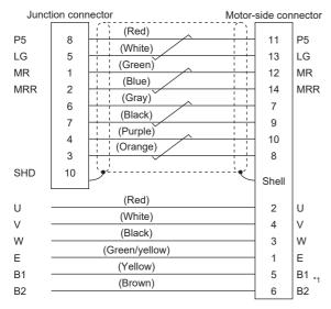
\*1 B1 and B2 are the wiring for electromagnetic brake. Wire when MR-AEPB2J20CBL03M-\_-L is used. If MR-AEP2J20CBL03M-\_-L is used, B1 and B2 do not need to be wired as MR-AEP2J20CBL03M-\_-L does not have B1 and B2.
