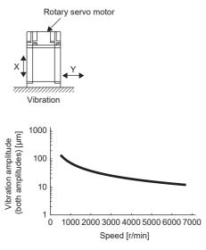
\*5 V10 indicates that the amplitude of a rotary servo motor as a single unit is 10 μm or less. The following figure shows the rotary servo motor mounting position for measurement and the measuring position.
