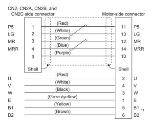
\*1 B1 and B2 are the wiring for electromagnetic brake. Wire when MR-AEPB2CBL\_M-\_- is used. If MR-AEP2CBL\_M-\_- is used, B1 and B2 do not need to be wired as MR-AEP2CBL\_M-\_- does not have B1 and B2.
