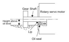
High pressure against the oil seal causes abrasion, which shortens the service life of the product. Keep constant internal pressure by equipping a ventilator to the gear box.
