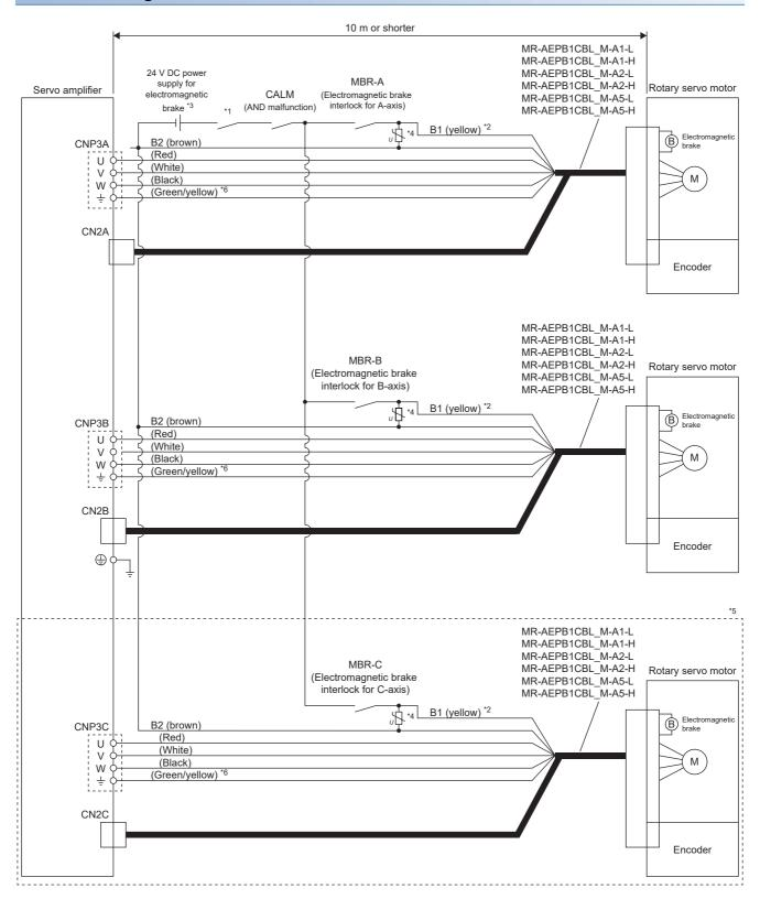
\*1 Configure a circuit which interlocks with an emergency stop switch to shut off.
