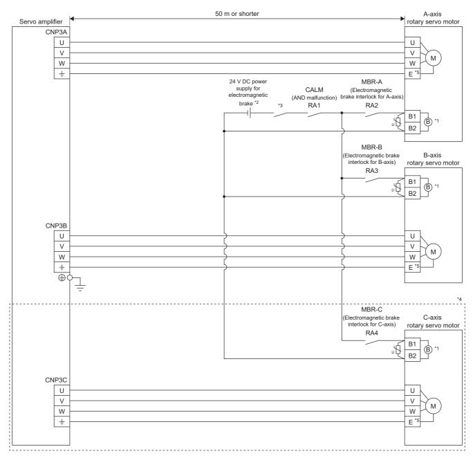
\*1 The electromagnetic brake terminals (B1 and B2) have no polarity.
