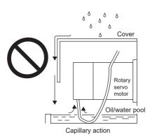
• When the servo motor is to be installed with the shaft end upward, provide measures so that it is not exposed to oil and water entering from the machine side, gear box, etc.
