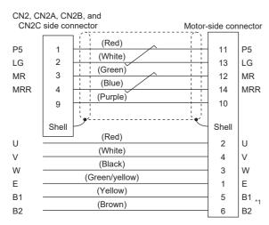
\*1 B1 and B2 are the wiring for electromagnetic brake. Wire when MR-AEPB1CBL\_M-\_- is used. If MR-AEP1CBL\_M-\_- is used, B1 and B2 do not need to be wired as MR-AEP1CBL\_M-\_- does not have B1 and B2.
