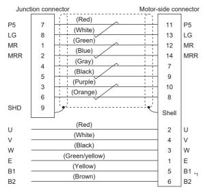
\*1 B1 and B2 are the wiring for electromagnetic brake. Wire when MR-AEPB2J10CBL03M-\_-L is used. If MR-AEP2J10CBL03M-\_-L is used, B1 and B2 do not need to be wired as MR-AEP2J10CBL03M-\_-L does not have B1 and B2.
