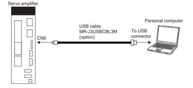
2. Start MR Configurator2 and create a new project. For the connection setting, select USB. Select the servo amplifier model.
