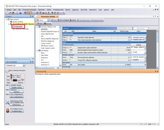
**6.** Select a group of servo parameters in the selection tree of the "Parameter Setting" window to display and configure the settings.
