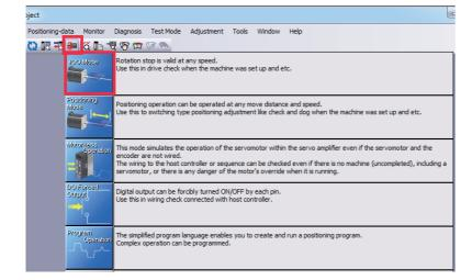
**5.** To operate the servo motor, input the motor speed and acceleration/deceleration time constants, then click "Forward CCW" or "Reverse CW". The servo motor operates only while the button is being clicked. Give a low speed command at first and check the operation status.
