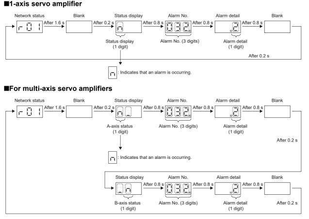
When a 3-axis servo amplifier is used, the alarm occurrence status in the B-axis is indicated before the alarm occurrence in the C-axis.
