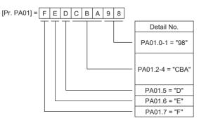
For example, if the servo parameter name is "Function selection A-1", the setting digit name is "Forced stop deceleration function selection", and the setting digit is the fourth last digit in PA04, the servo parameter is expressed as shown below. [Pr. PA04.3 Forced stop deceleration function selection]
