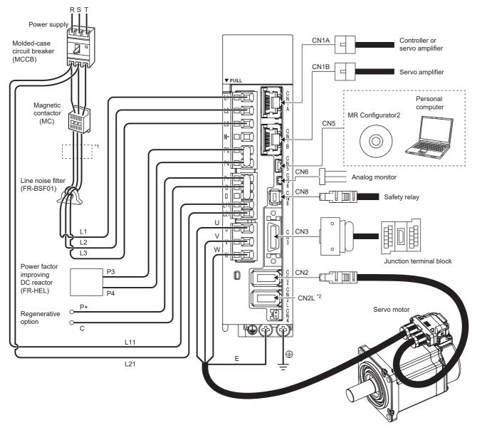
\*1 The power factor improving AC reactor can also be used. In this case, the power factor improving DC reactor cannot be used.
