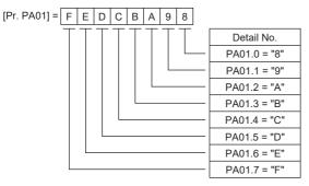
· When setting a servo parameter using a combination of several digits
