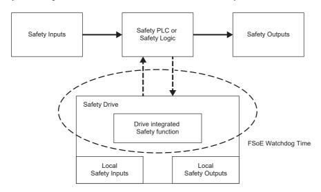
TRef + TCom × 4 = 16 (Unit: ms) is the minimum configurable value for FSoE Watchdog Time.
