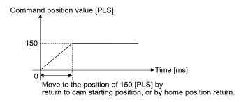
• Restore operation at start of synchronous control
