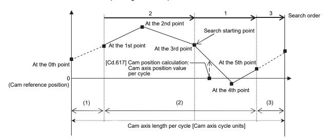
Example) When "[Cd.617] Cam position calculation: Cam axis position value per cycle" is corresponding to the 3rd point of cam data
