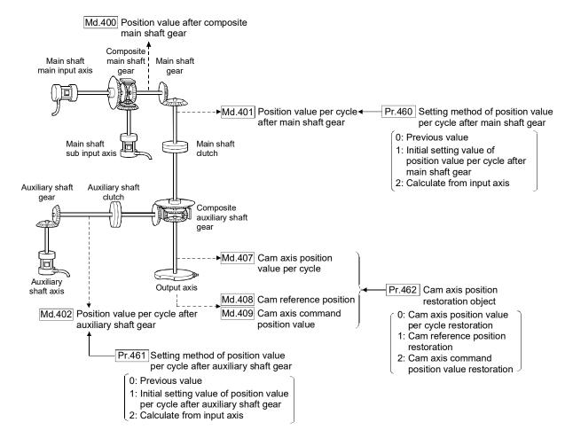
■ Position value after composite main shaft gear when starting synchronous control The position value after composite main shaft gear is restored as follows according to the main input axis operation executed before starting synchronous control.
