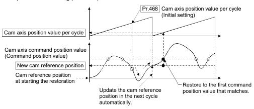
(c) Search from a value in the middle of the cam axis position value per cycle. (Cam data starting point ≠ 0)
