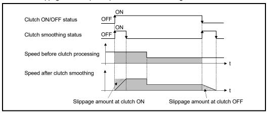
When the input speed to the clutch is changed continuously and slightly The clutch smoothing status ON section is changed.
