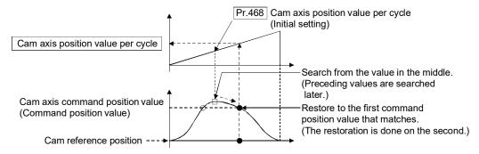
(c) Search from a value in the middle of the cam axis position value per cycle.
