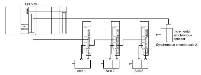
Set "1: Incremental synchronous encoder" in "[Pr.320] Synchronous encoder axis type" for the synchronous encoder axis 2.
