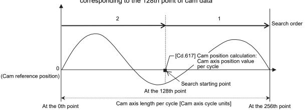
Searches until between the 255th point and the 256th point (last point) in order of the cam data between the 128th point and the 129th point and between the 130th point and the 131st point.
