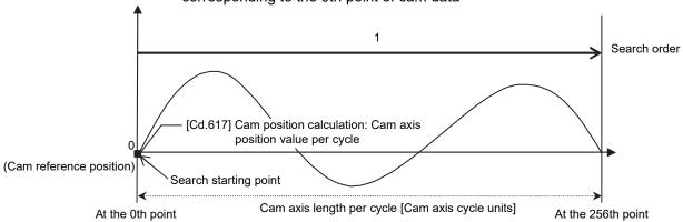
• Searches until between the 255th point and the 256th point (last point) in order of the cam data between the 0th point and the 1st point and between the 1st point and the 2nd point.
