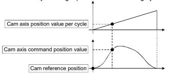
Select from 3 objects as follows in "[Pr.462] Cam axis position restoration object" which position is to be restored.
