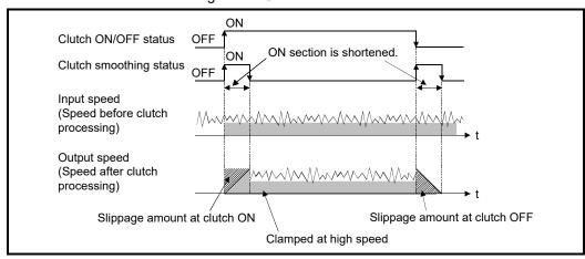
• When the input speed is changed largely during smoothing
