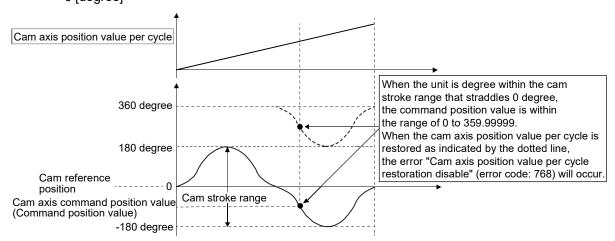
Restore the position value within the cam stroke range that is out of the range of 0 to 360 [degree].
