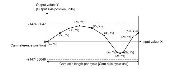
When an input value that is 0 or the cam axis length per cycle does not exist in the coordinate data, the coordinate is calculated from the line segment between the nearest two coordinates.
