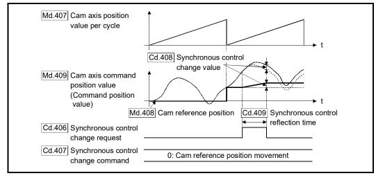
When "[Cd.406] Synchronous control change request" is reset to "0" while executing the cam reference position movement command, operation is stopped midway. If the cam reference position movement command is executed again, the remainder travel value is not reflected, and the operation starts with "[Cd.408] Synchronous control change value" to be used again.
