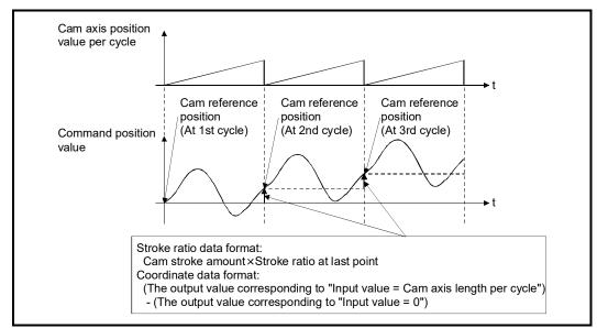
Create cam data for two-way cam operation as shown below.
