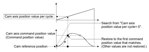
(b) Search from a value in the middle of the cam axis position value per cycle. (Cam data starting point = 0)
