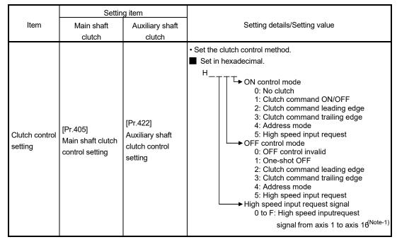
(Note-1): The range from axis 1 to 2 is valid in the 2-axis module, from axis 1 to 4 is valid in the 4-axis module, from axis 1 to 8 is valid in the 8-axis module, and from axis 1 to 16 is valid in the 16-axis module.
