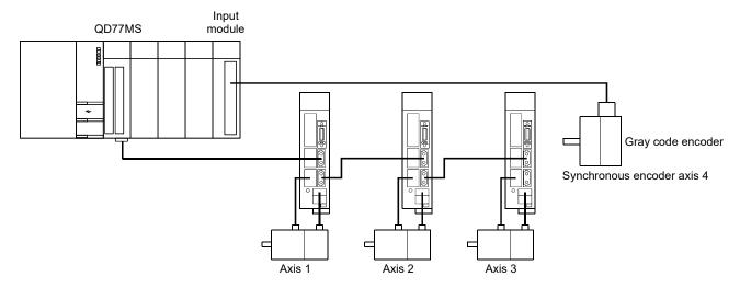
Set "201: Synchronous encoder via CPU" in "[Pr.320] Synchronous encoder axis type" of synchronous encoder axis 4.
