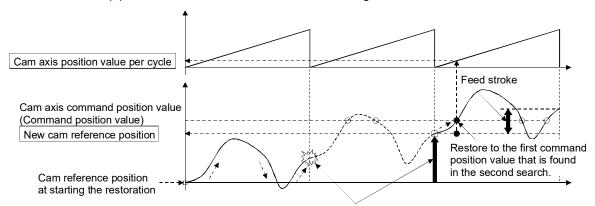
Once the restoration fails in the first search, the new cam reference position is automatically updated to set "Command position value - New cam reference position" to be within the feed stroke amount, and the search process starts again.
