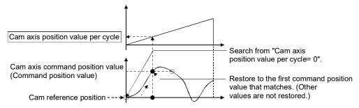
(b) Search from a value in the middle of the cam axis position value per cycle. (Cam data starting point = 0)
