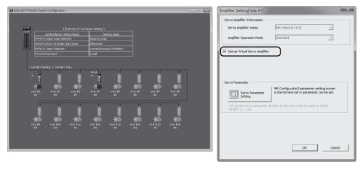
2) Set the axis 4 as the servo input axis in the input axis parameter.
